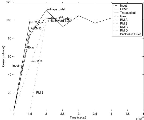
Fig. 4 Step Response with 500  $\mu$ sec time-step
