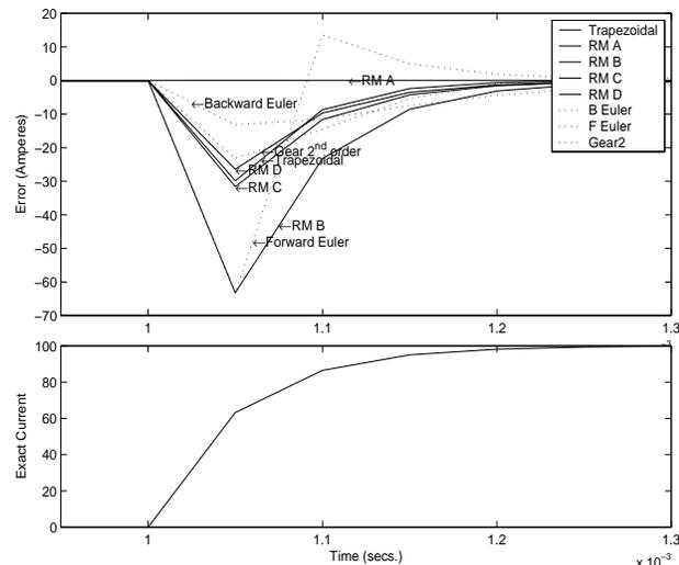
Fig. 5 Step Response with 50  $\mu$ sec time-step
