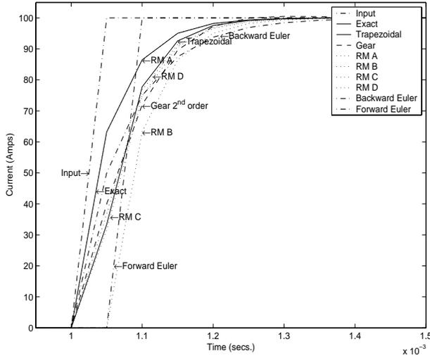
Fig. 3 Step Response with 50  $\mu$ sec time-step
