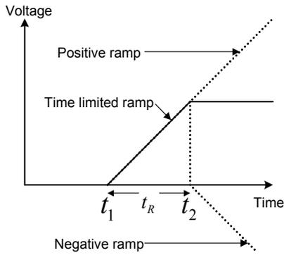
Fig. 6 Time Limited Ramp Input
