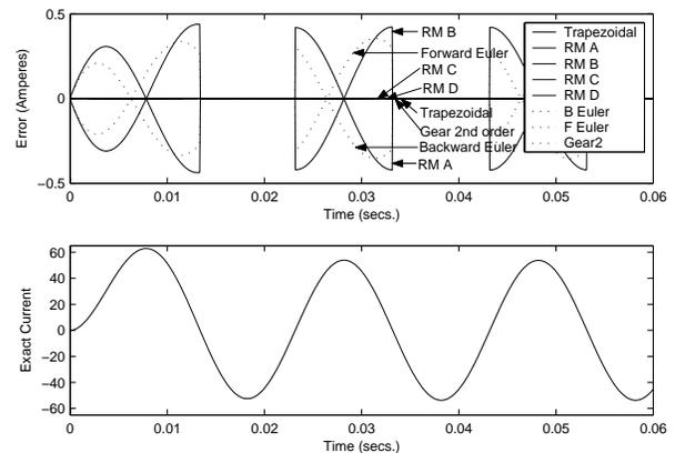
Fig. 14 Error in Switched Sinusoid Simulation
