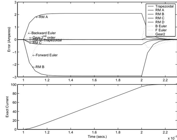
Fig. 8 Error for a 1 msec ramp Input
