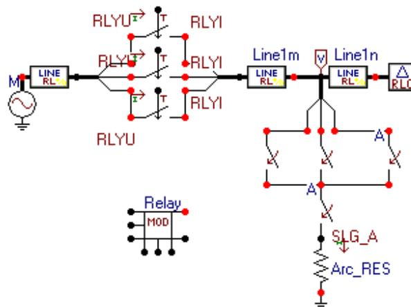
Fig. 7 Distribution network for ATP simulation
