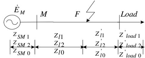
Fig. 1 Single source line with load
