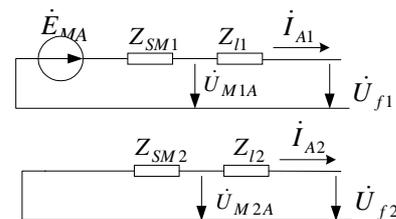
Fig. 4 Fault-condition sequence network of system in Fig.3
