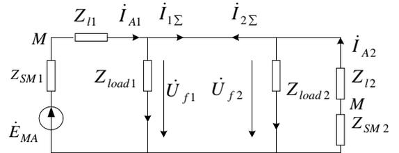
Fig. 2. Sequence network under fault status of system in Fig. 1
