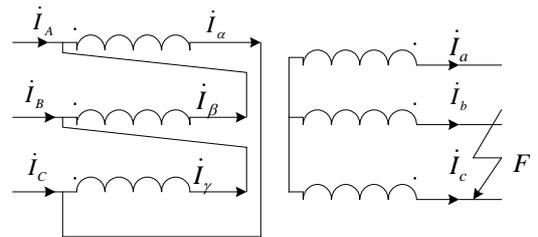
Fig. 5 Distribution of primary and secondary currents of transformer
