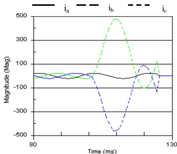
Fig.8 Phase currents when B-C phase fault occurs
