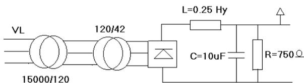
Fig. 3 Rectifier and filter
