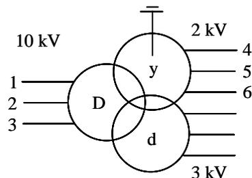
Fig. 2 3-winding transformer
