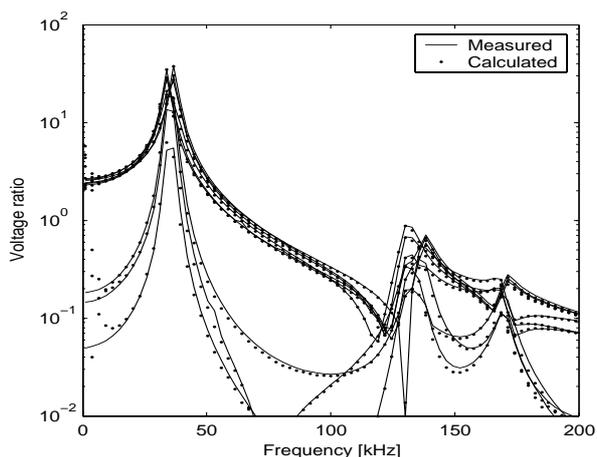
Fig. 6 Voltage ratio from low to high ( $V_{HL}$ )
