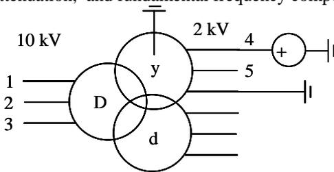
Fig. 11 Excitation of low voltage winding
