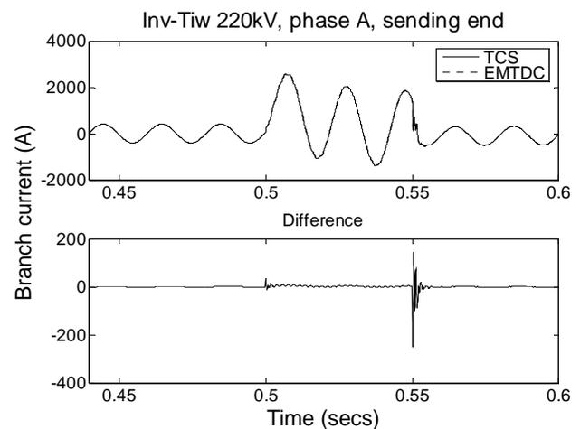
Fig. 13. Sending end Invercargill-Tiwai branch current, phase A
