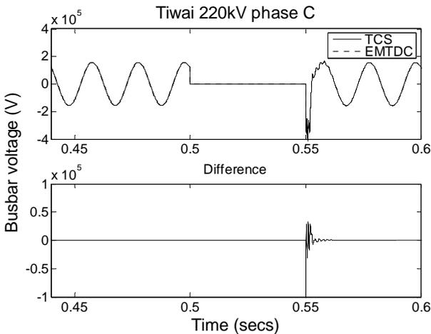
Fig. 4. Busbar voltage at Tiwai 220kV phase C
