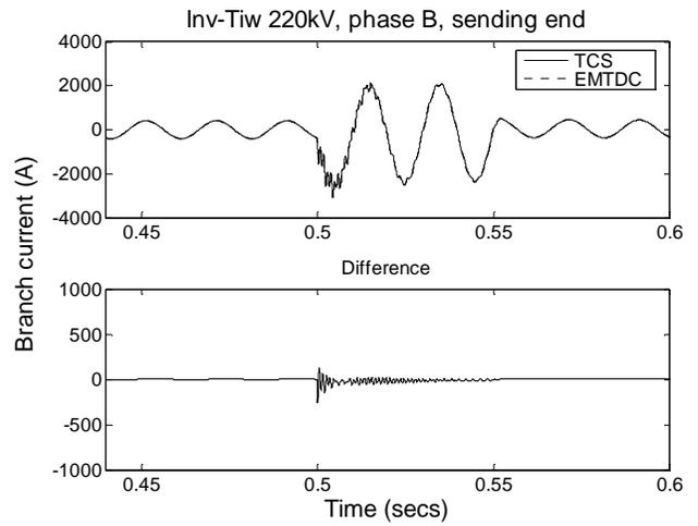
Fig. 6. Sending end Invercargill-Tiwai branch current, phase B
