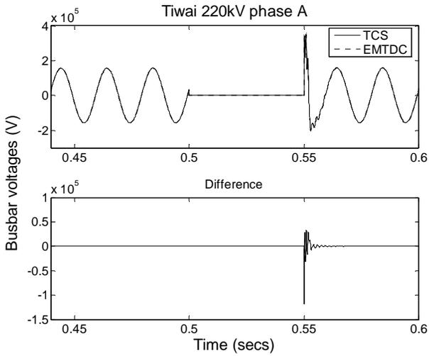
Fig. 2. Busbar voltage at Tiwai 220kV phase A
