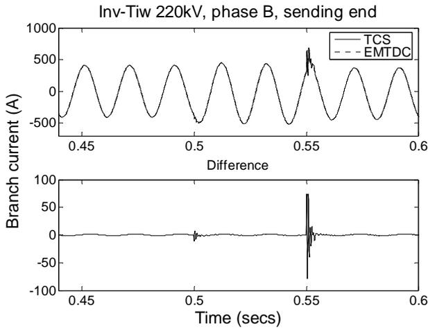
Fig. 14. Sending end Invercargill-Tiwai branch current, phase B
