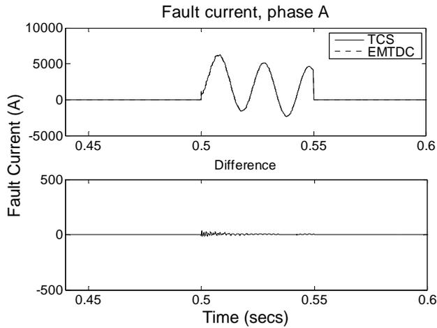
Fig. 8. Fault current, phase A
