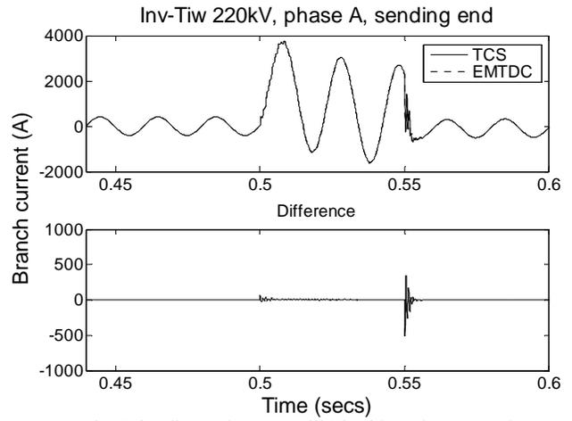
Fig. 5. Sending end Invercargill-Tiwai branch current, phase A
