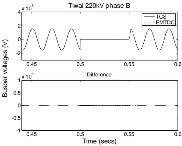
Fig. 3. Busbar voltage at Tiwai 220kV phase B
