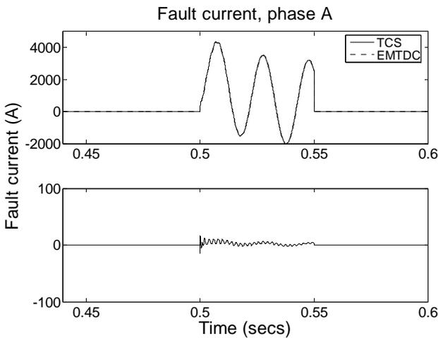
Fig. 15. Fault current, phase A
