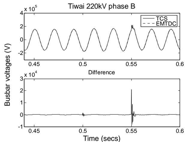
Fig. 12. Busbar voltage at Tiwai 220kV phase B
