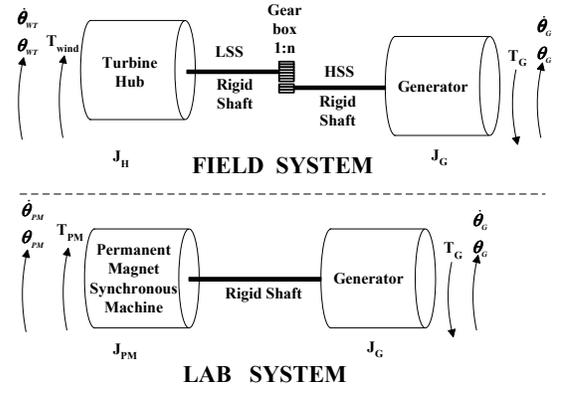
Fig. 4. Mechanical diagram of field system (with rigid LSS and rigid HSS) and lab system
