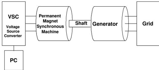
Fig. 2. Lab System: Simplified Diagram of Wind Turbine Emulator - The lab system is realized by replacing the wind and rotor of the field system with a PC, VSC and PMSM
