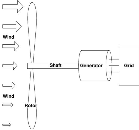
Fig. 1. Field System: Simplified Diagram of Modelled Wind Turbine System
