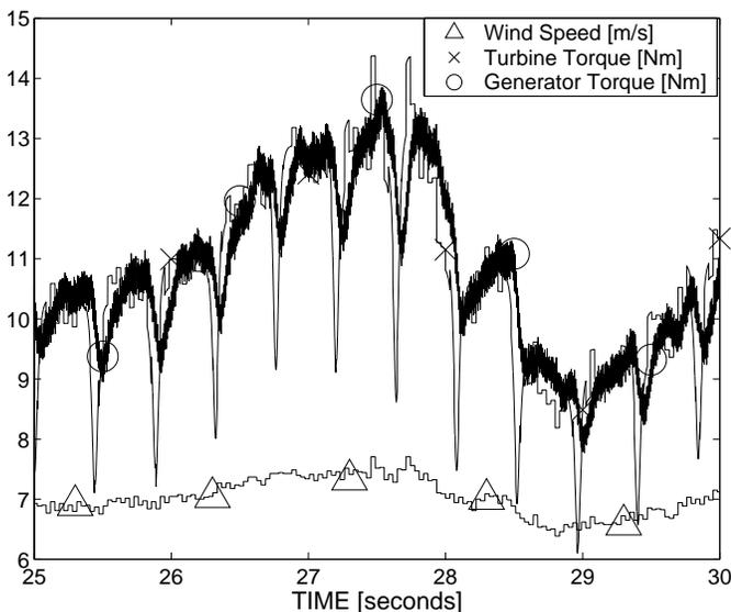
Fig. 9. Generator Torque including effects of Tower Shadow, Wind Shear and inertia 23 times larger than generator
