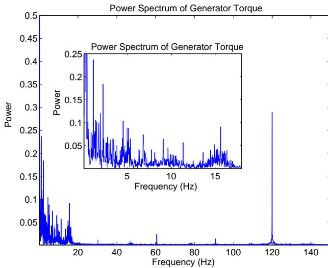
Fig. 8. Frequency spectrum of the generator torque for 6% tower shadow induced torque oscillation without inertial effects
