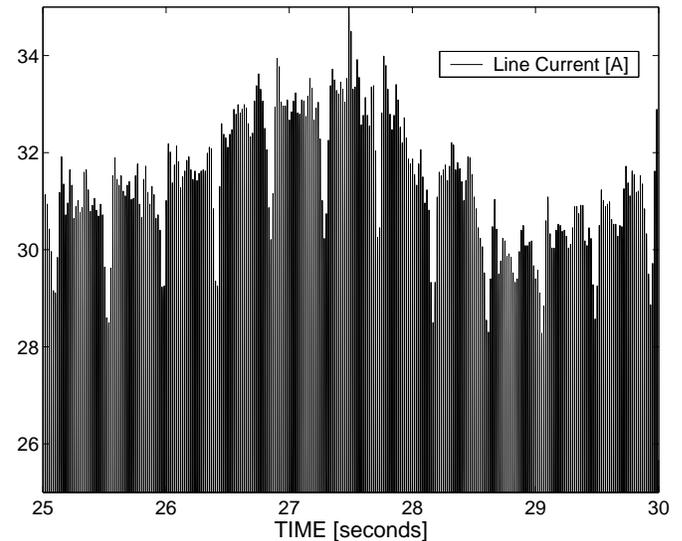
Fig. 7. Line current from generator showing depressions due to Tower shadow effect and variations due to changing wind speeds
