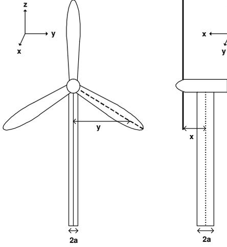
Fig. 3. Dimensions used in tower shadow formula
