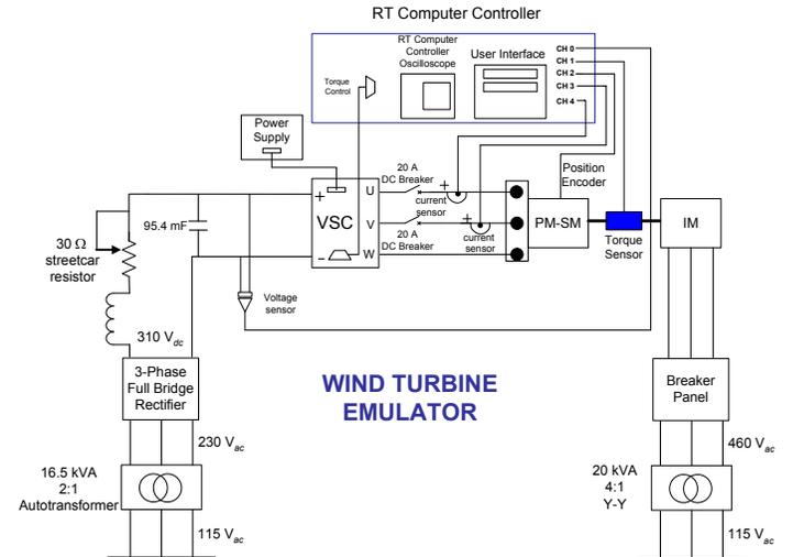
Fig. 5. Wind Turbine Emulator: Experimental Setup
