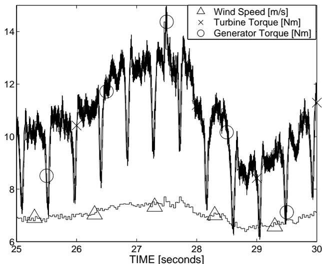
Fig. 6. Generator Torque including only effects of Tower Shadow and Wind Shear
