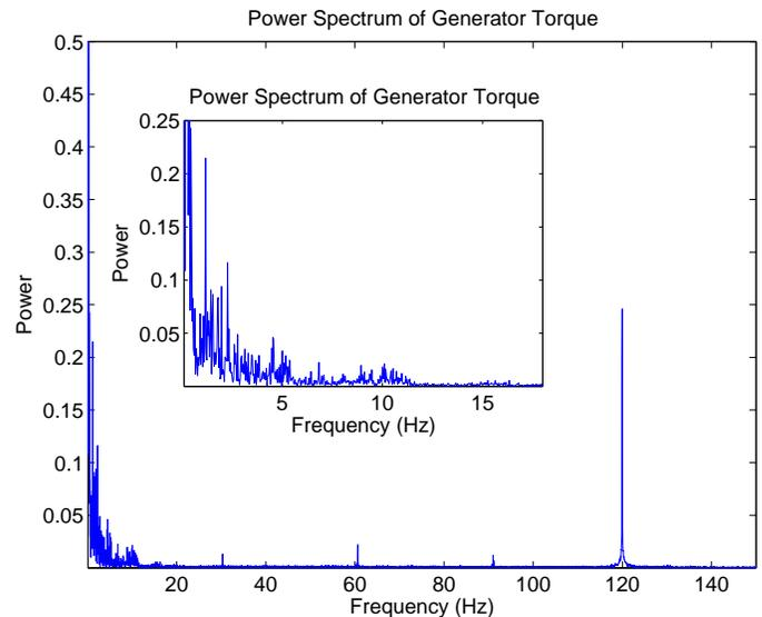
Fig. 11. Frequency spectrum of the generator torque for 6% tower shadow induced torque oscillation with inertial effects included
