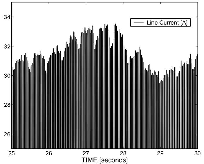
Fig. 10. Line current from generator showing depressions due to Tower shadow effect and variations due to changing wind speeds smoothed by large turbine inertia
