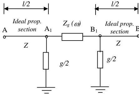
Fig. 1 - Grounding conductor segment
