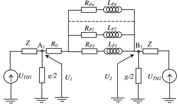
Fig. 3 - Equivalent circuit for determination of the voltages in middle of the segment
