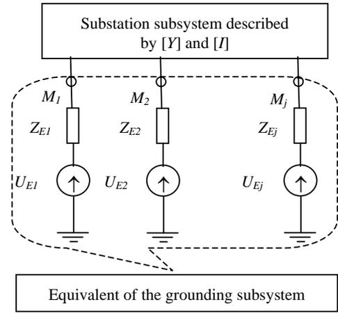
Fig. 4 – Interconnection of the substation and the grounding subsystems
