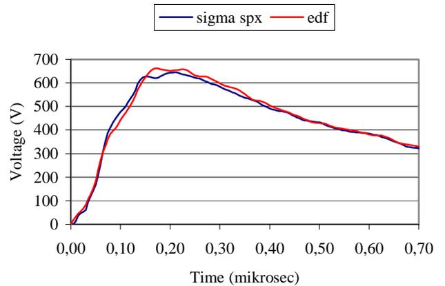
Fig. 6 - Voltage shapes at the injection point (15 m grounding conductor)
