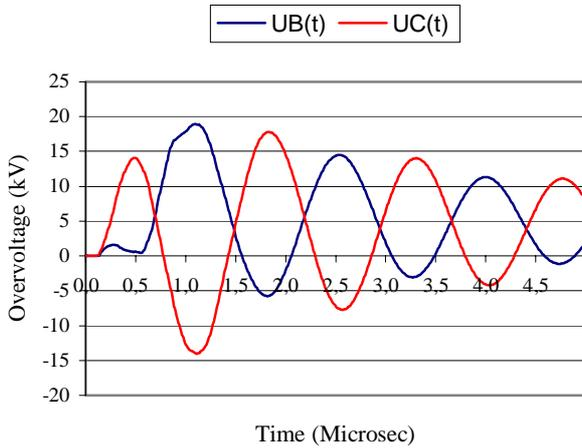
Fig. 10 - Overvoltage shapes at the SSA and PT grounding nodes (Nodes B and C)
