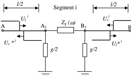
Fig. 2 - Traveling waves on the conductor segment
