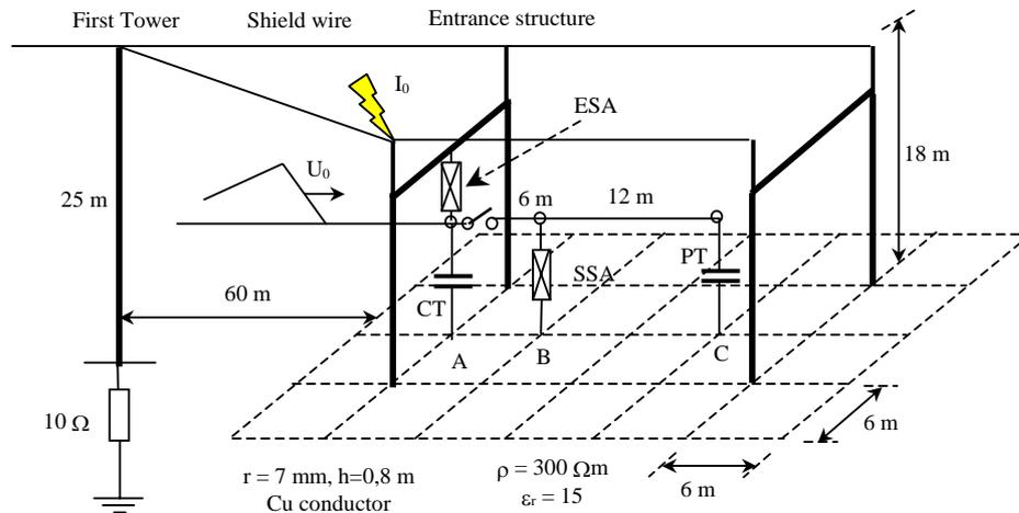
Fig. 8 - 123 kV High voltage substation
