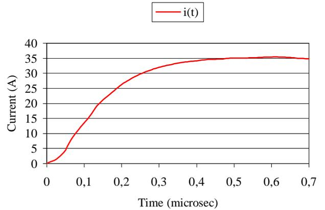
Fig. 5 - Impulse current used in the EdF experiment
