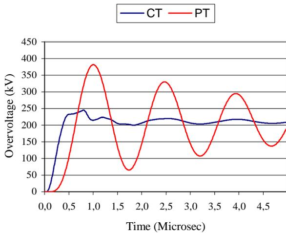
Fig. 9 - Overvoltage shapes on the current transformer and on the power transformer
