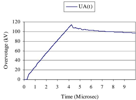
Fig. 11 - Overvoltage shapes at the current transformer grounding side (Node A) Stroke hits lightning protection system
