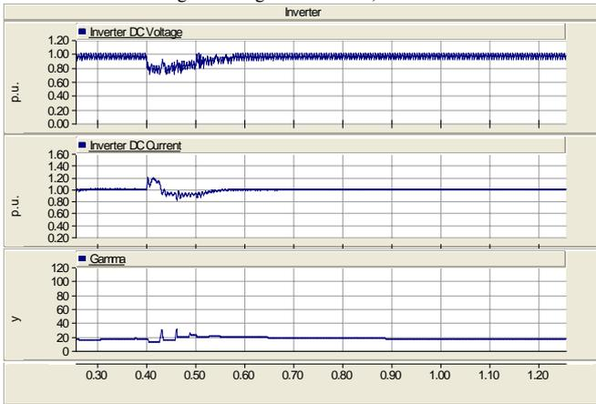
Fig. 5. Three Phase Fault,  $R_f=90\Omega$
