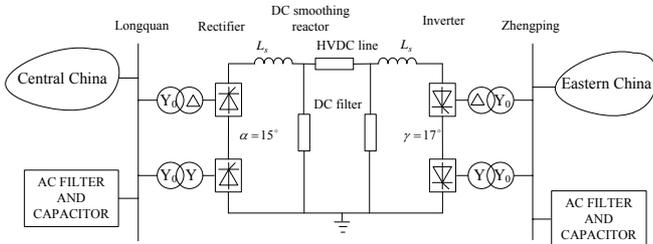
Fig. 3. Monopolar of Longquan-Zhengping HVDC Link
