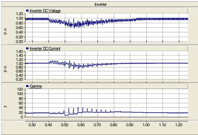
Fig. 4. Single Phase Fault,  $R_f=90\Omega$
