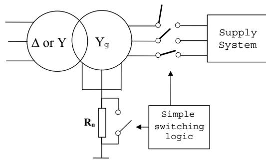
Fig. 1 The sequential phase energization inrush mitigation technique.
