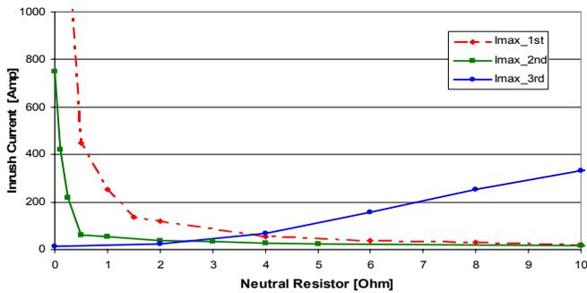
Fig. 2 Magnitude of inrush current as affected by the neutral resistor for a 30kVA, 208/208, Yg- $\Delta$ , 3 limb transformer. (Experimental)
