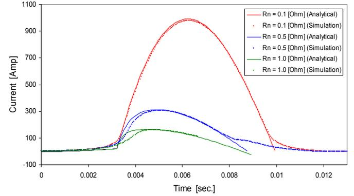
Fig. 5 Analytical and simulation inrush current waveforms (first cycle) for 30kVA Yg-Δ transformer.
