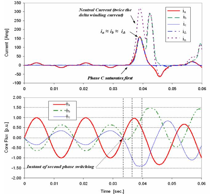
Fig. 7 Simulation of the 30kVA transformer during second phase switching condition showing the phase fluxes and effect of Delta winding current for small values of  $R_n = 0.1$  [Ohm].
