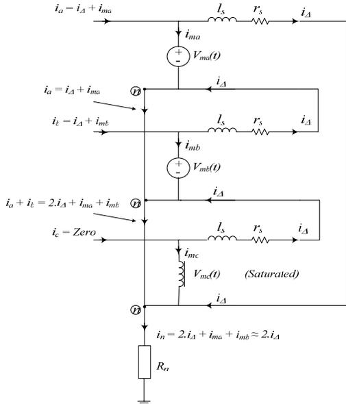
Fig. 8 Modeling the delta winding during saturation condition of phase C.
