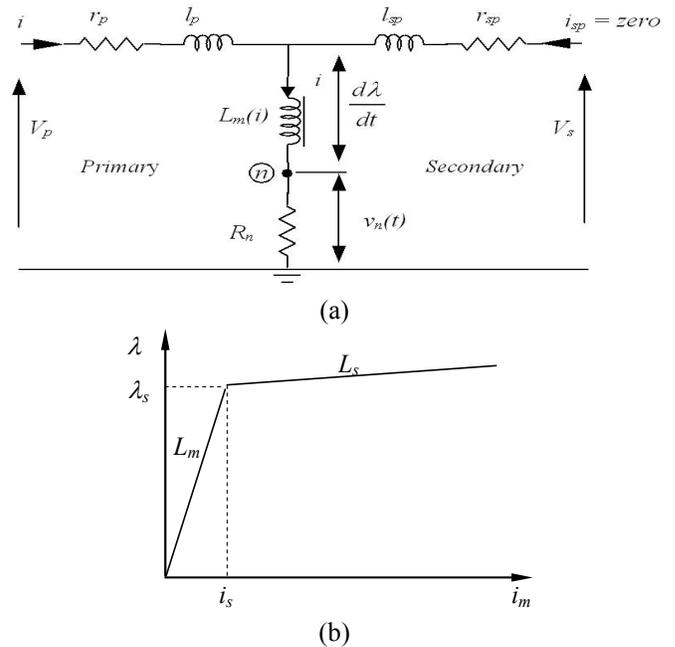
Fig. 4 (a) Transformer electrical equivalent circuit (per-phase) referred to the primary side. (b) Simplified, two sloped saturation curve.
