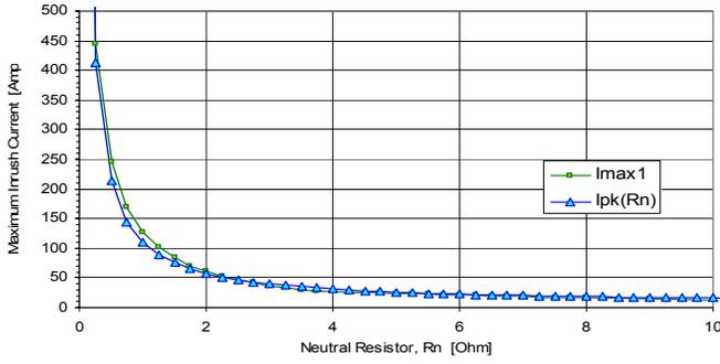
Fig. 6.  $I_{pk}(R_n)$  compared to the simulation peak current for 30 kVA, 208/208 Yg- $\Delta$ , three limb transformer.
