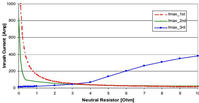
Fig. 3 Maximum inrush current as affected by the neutral resistor for a 30kVA, 208/208, Yg-D, 3 Limb transformer. (Simulation)
