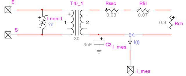
Fig. 3. CT modeling.  $R_{sec}$ ,  $R_{fil}$  and  $R_{ch}$  are respectively the secondary winding, cable link and charge resistances (values are in ohms). The total resistance is  $R_t = R_{sec} + R_{fil} + R_{ch} = 1.0 \Omega$
