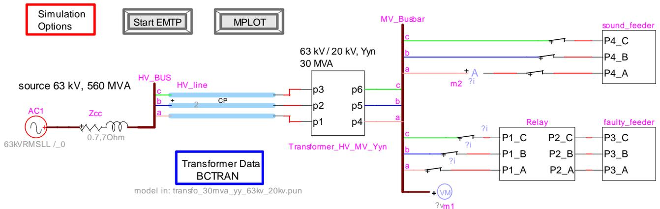
Fig. 1. Radial MV network fed by a HV line through a 30 MVA transformer. The studied relay protects the faulty feeder.
