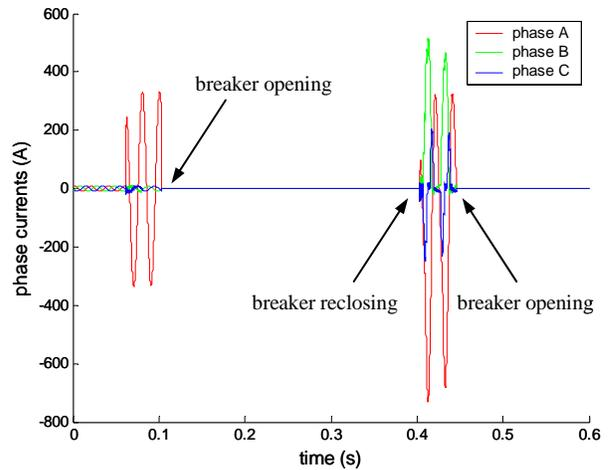
Fig. 9. Phase currents for a reclosing sequence with a permanent fault
