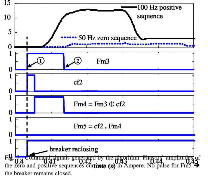
Fig. 5. Command signals generated by the algorithm. Phase's amplitudes of the zero and positive sequences current (time (s)) in Ampere. No pulse for Fm5 → the breaker remains closed.
