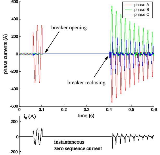
Fig. 6. Phase currents for a reclosing sequence with a transient fault.
