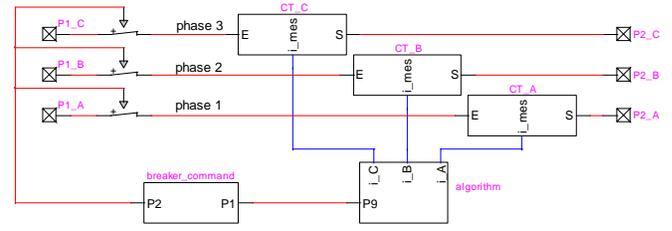
Fig. 2. Protective relay with the three CTs, the algorithm and the breaker's command.
