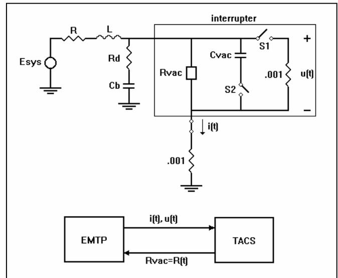
**Figure 3. Circuit diagram for the simulation of a breaker terminal fault and block diagram showing the flow of variables between ATP and TACS.**
