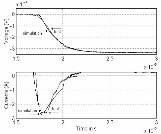
**Figure 4** Traces for comparison of test with simulation, after use of the extracted constants from the parameter extraction and optimization program.
