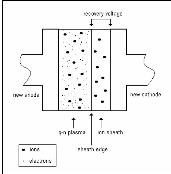
**Figure 2. Visualization of sheath development during post-arc period.**
