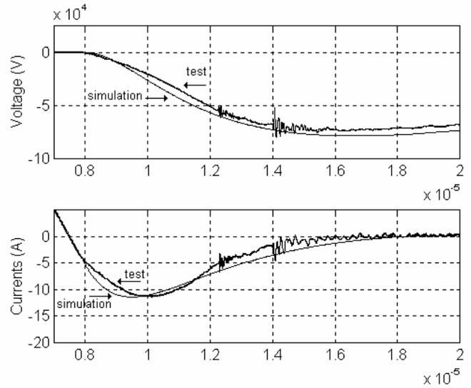
**Figure 5** Other traces for comparison of test with simulation, after use of the extracted constants from the parameter estimation program.
