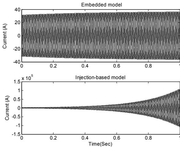
Fig. 10. Armature currents of the machines in time step  $167 \mu S$
