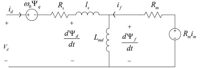
Fig. 4. D axis thevenin equivalent circuit of the PMSM
