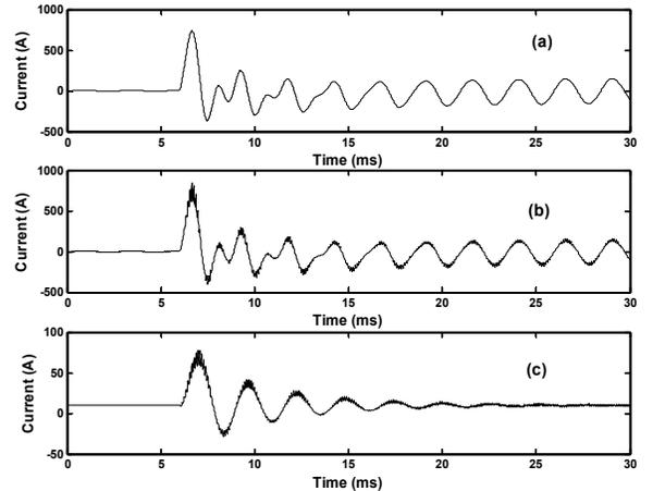
Fig. 13. The currents of the machine in short circuit a) phase current of dq0 model of the machine b) phase current of embedded model of the machine c) Field current of embedded model of the machine
