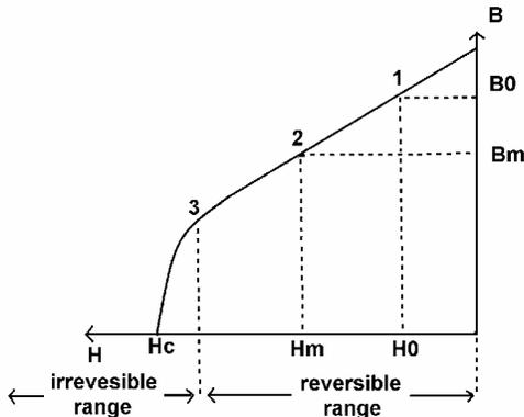
Fig. 3. Demagnetization curve of the permanent magnet [4]
