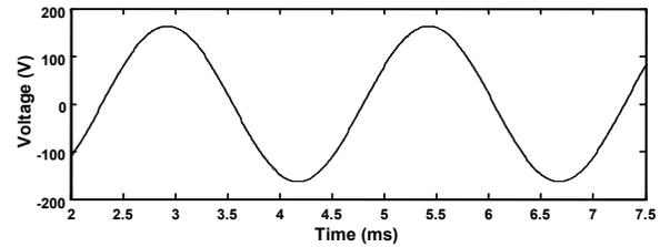
Fig. 12. Phase A open circuit voltages of the machines
