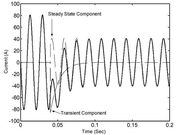
Fig. 9. Three phase short circuit current of the machines
