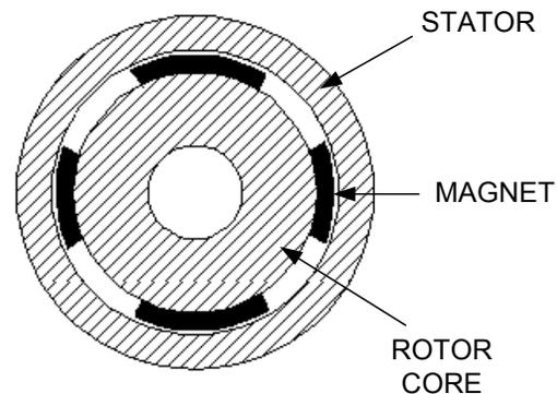
Fig. 1. Structure of the permanent magnet synchronous machine [3]
