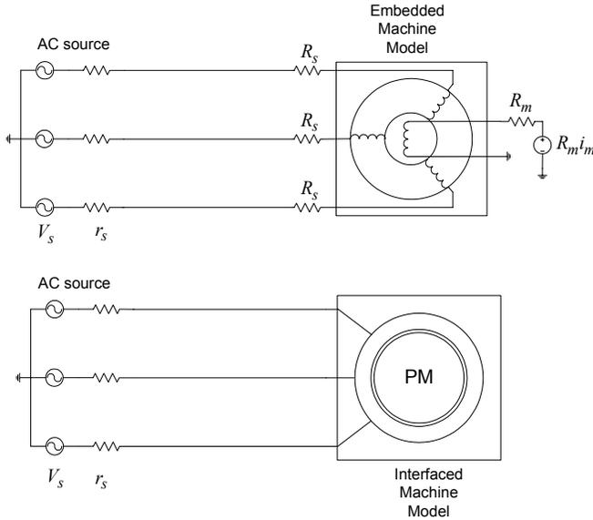
Fig. 6. Test circuit for comparing the new machine models
