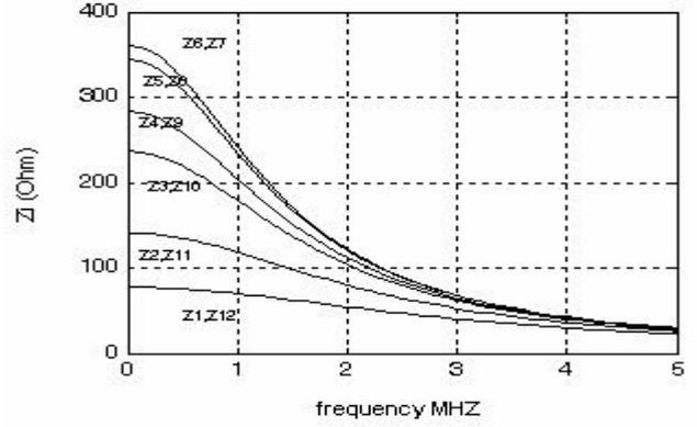
Fig. 3: Characteristic impedance of discs as a function of frequency ( $i=1, \dots, 12$ )
