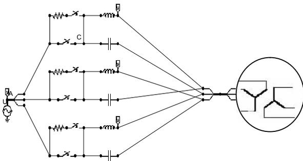
Fig. 6: In time domain simulated IPC with the transformer is modeled with MTLT and the sinusoidal power supply is shown (Inductances are 110 mH and capacitances are 0.12 F)
