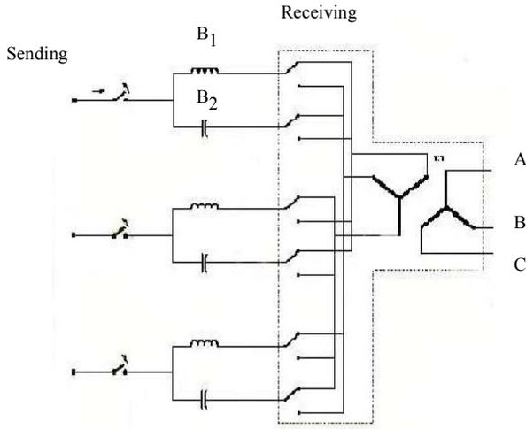
Fig. 2 : Schematic diagram of the typical IPC120
