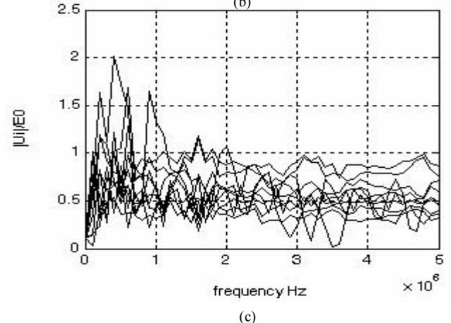
Fig. 4: Ratio of inter-discs voltage to its input voltage,
