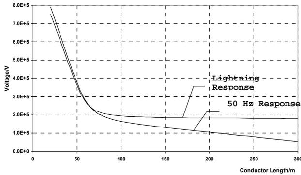
Fig. 3. Max Ground Potential rise values vs. conductor length
