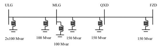
Figure 4 - Reactive compensation for the expanded bundle configuration
