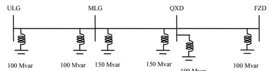
Figure 3 - Reactive compensation for the standard bundle configuration
