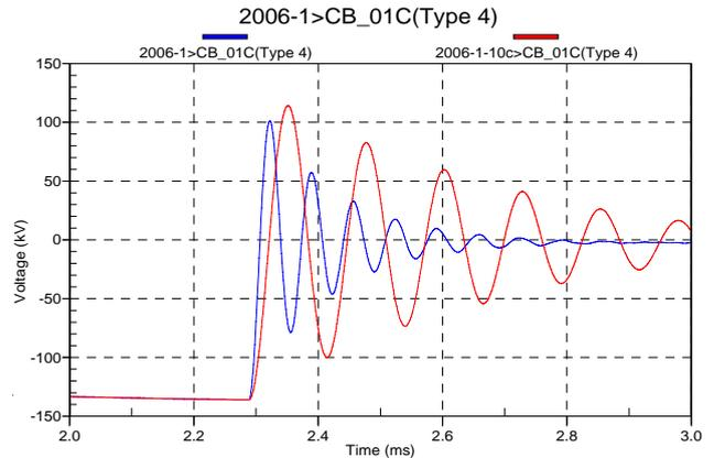
Comparison - Before and After Installing 20000pF capacitor in circuit breaker on both sides of 345kV T/L
