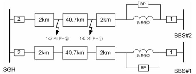
Fig. 2 - Simulation Condition on T/L
