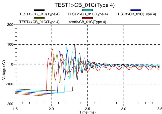
Fig. 4 RRRV waveform by distance at SLF
