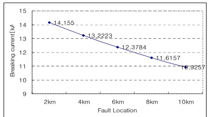
Fig. 6 - Breaking current by distance at SLF
