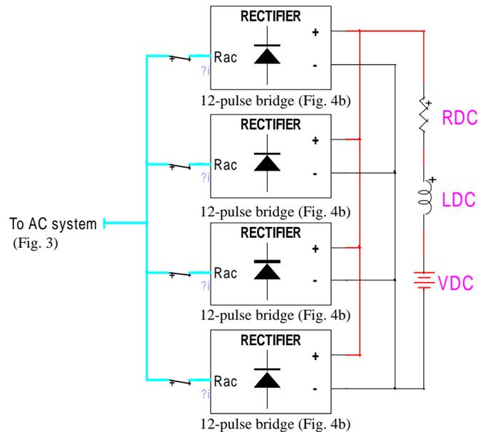
Fig. 4a. 48-pulse rectifier load modeling (EMTP-RV)
