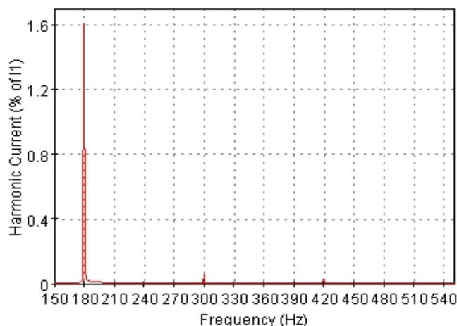
Fig. 1. Harmonic content of network current under voltage unbalance for near idealized conditions (DFT analysis) of a 48-pulse rectifier load
