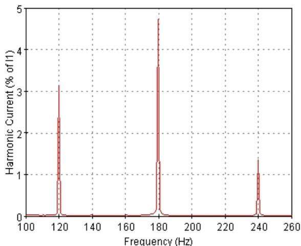
Fig. 10. Harmonic content of network current waveform under unbalanced voltages and saturable reactor asymmetrical characteristics (DFT analysis)
