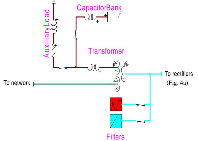
Fig. 3. AC system modeling (EMTP-RV)
