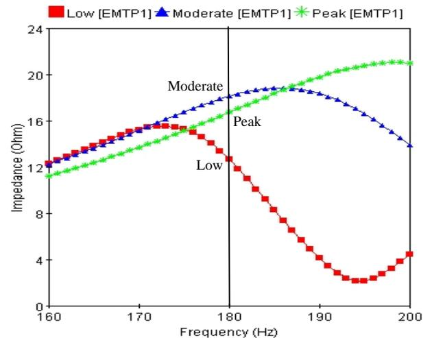
Fig. 8. Proposed model frequency scan
