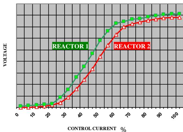
Fig. 9. Asymmetrical characteristic of two saturable reactors
