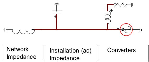
Fig. 6. Proposed model for low-order non-characteristic harmonics
