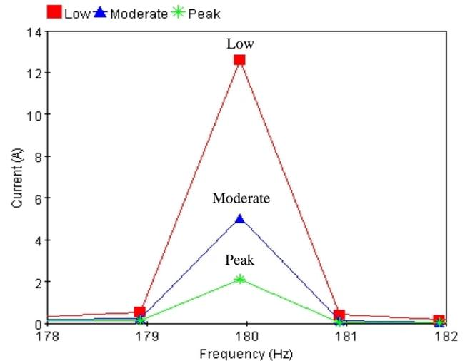
Fig. 5. Discrete Fourier Transform (DFT) analysis of the third harmonic current generated by one rectifier
