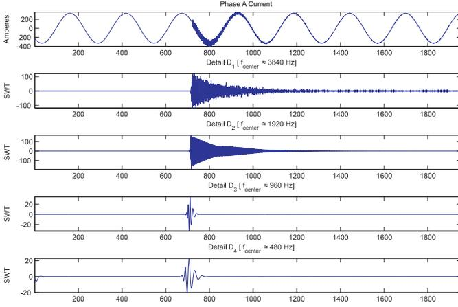
Fig. 6. SWT details during fault occurrence.
