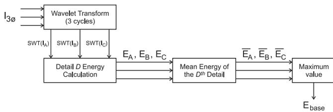
Fig. 3. Base Characteristics Extraction.
