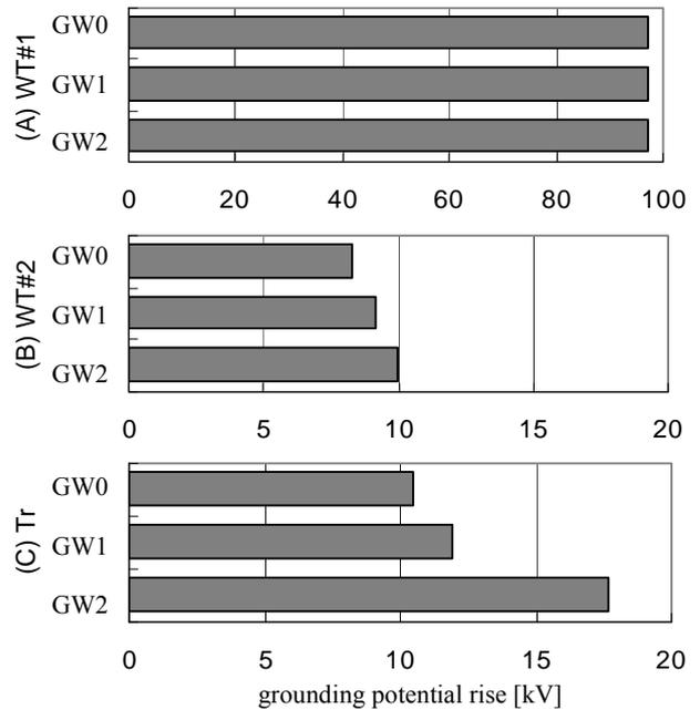
Fig.8. Maximum grounding potential rise at points around the wind farm in case of summer lightning ( $2/70 \mu\text{s}$ , 30 kA)
