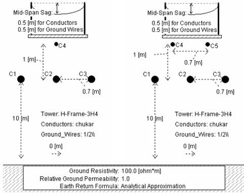
Fig. 4 Distribution line model in wind farm (by PSCAD description) (Left: 1-ground-wire model, Right: 2-ground-wires model)
