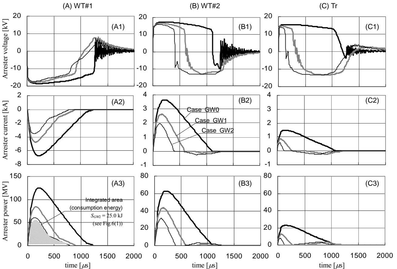
Fig. 6 Calculated waveforms at surge arresters at various points among the wind farm in case of summer lightning (2/631  $\mu$ s, 51 kA). (Column (A): wind turbine No.1 (WT#1), Column (B): wind turbine No.2 (WT#2), Column (C): grid-interactive transformer (Tr), Row (1): voltage between terminals of arrester, Row (2): current through arrester, Row (3): simultaneous power consumed at arrester)
