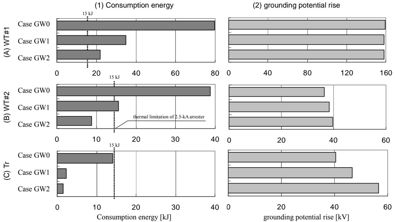
Fig.7. Energy consumption at surge arresters and maximum grounding potential rise at points around the wind farm in case of summer lightning ( $2/631 \mu\text{s}$ , 51 kA). (Column 1: total consumption energy at arrester, Column 2: maximum grounding potential rise, Row A: wind turbine No.1 (WT#1), Row B: wind turbine No.2 (WT#2), Row C: grid-interactive transformer (Tr).)
