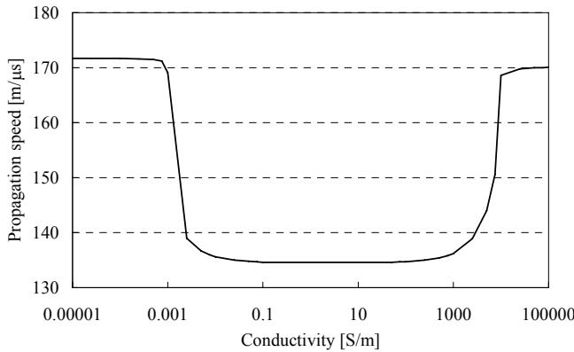
Fig. 3. Dependence of the propagation speed of a 30-MHz signal on the semiconducting-layer conductivity  $\sigma$ .
