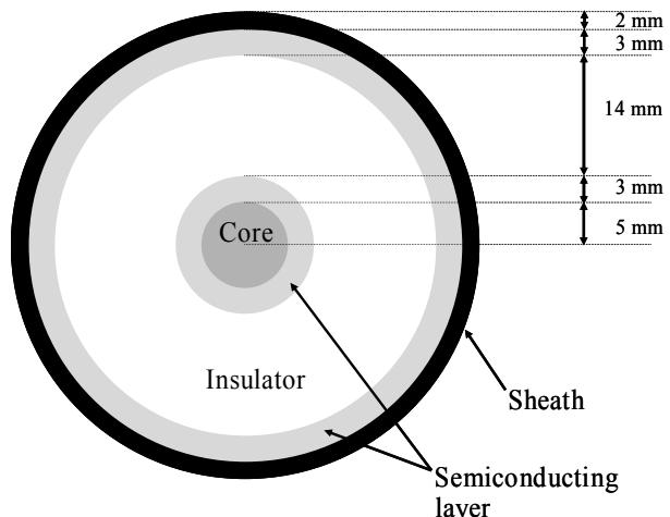
Fig. 1. Cross-section of a 130-m long single-core power cable, to be analyzed using the FDTD method.
