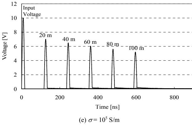
Fig. 2. Waveforms of the voltage between the core and the sheath conductor at different distances from the excitation point when the signal frequency is  $f=30$  MHz and the semiconducting-layer conductivity is  $\sigma=10^{-5}$ ,  $10^{-3}$ ,  $1$ ,  $10^3$ , and  $10^5$  S/m.
