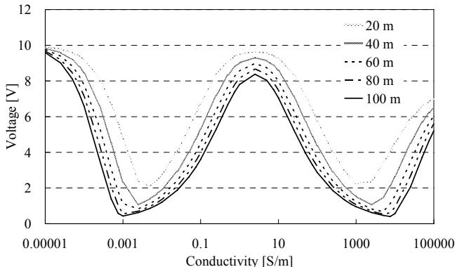
Fig. 4. Dependences of the magnitude of the voltage between the core and the sheath conductor at different points on the semiconducting-layer conductivity  $\sigma$ .
