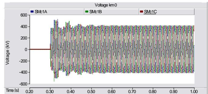
Fig. 8. Voltage at Serra da Mesa – km 0 – Complete simulation – Without pre-insertion resistor
