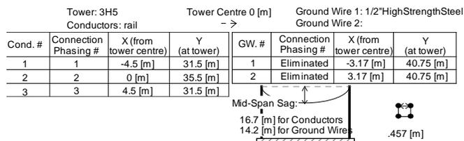
Fig. 4. N-S I towers data – phase conductor : rail
