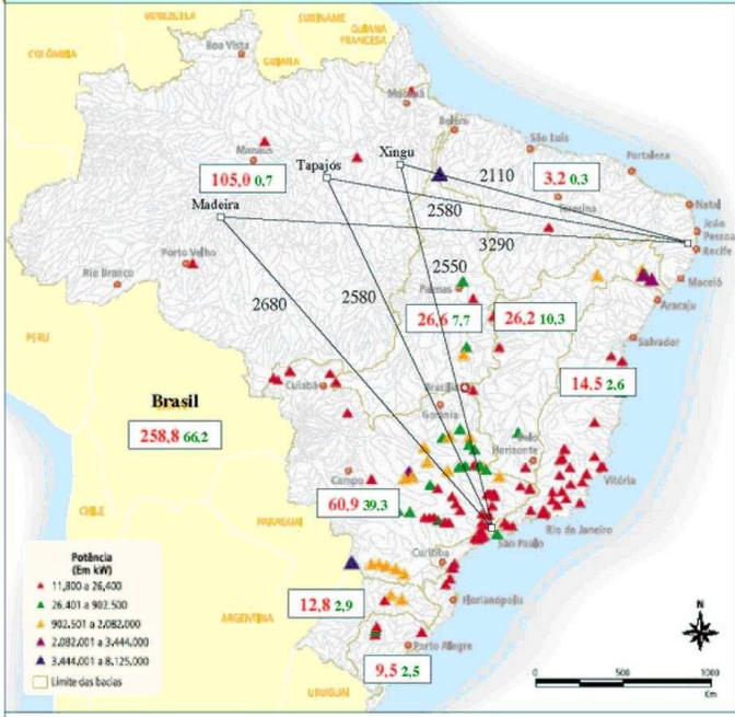
Fig. 3. Basic transmission distances from new Amazon plants and load centers – Distances in km; installed power and power capacity in GW
