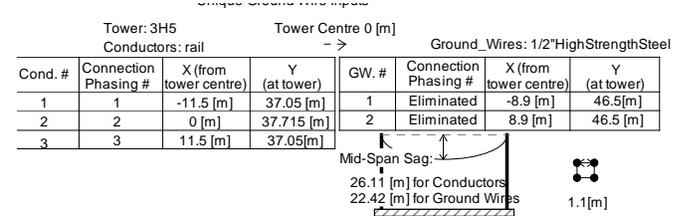
Fig. 6. NE-SE towers data – phase conductor : rail
