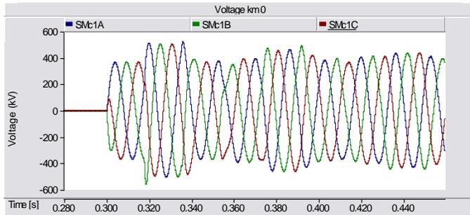
Fig. 11. Voltage at Serra da Mesa – km 0 – Simulation detail – Without pre-insertion resistor
