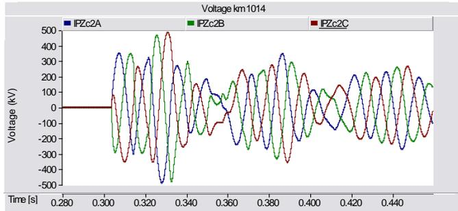
Fig. 12. Voltage at Imperatriz – km 1014 – Simulation detail – Without pre-insertion resistor
