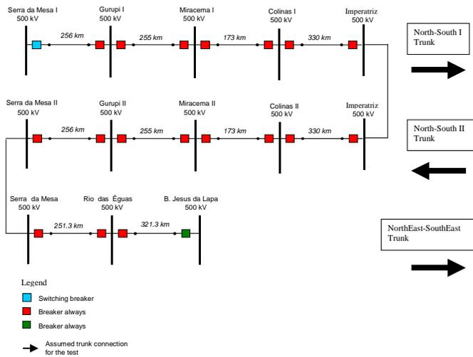
Fig. 7. AC-link 500 kV “test line” single phase diagram
