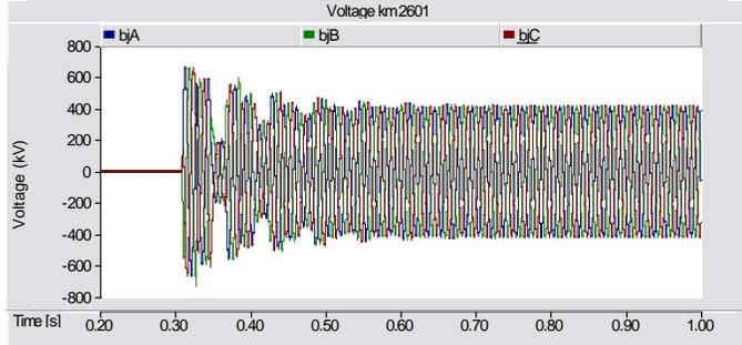
Fig. 10. Voltage at Bom Jesus da Lapa – km 2601 – Complete simulation Without pre-insertion resistor
