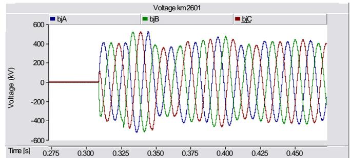
Fig. 17. Voltage at Bom Jesus da Lapa – km 2601 – Simulation detail – 140 Ω pre-insertion resistor
