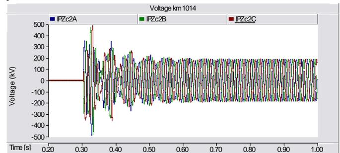
Fig. 9. Voltage at Imperatriz – km 1014 – Complete simulation – Without pre-insertion resistor
