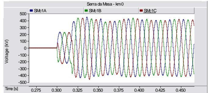
Fig. 16. Voltage at Serra da Mesa – km 0 – Simulation detail – 140 Ω pre-insertion resistor
