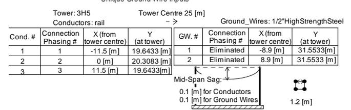
Fig. 5. N-S II towers data – phase conductor : rail
