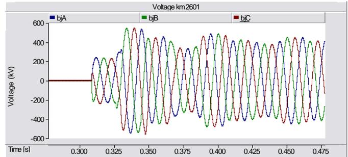
Fig. 15. Voltage at Bom Jesus da Lapa – km 2601 – Simulation detail – 400 Ω pre-insertion resistor
