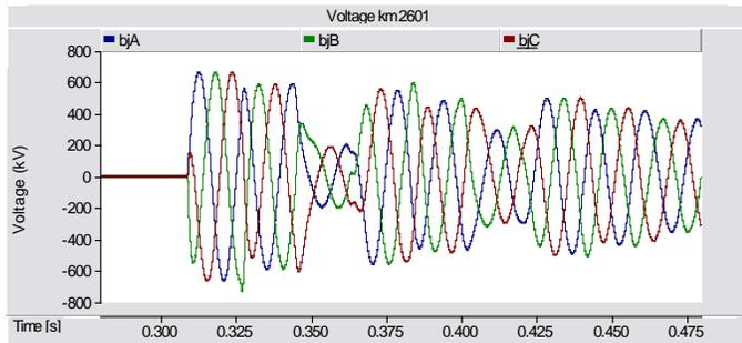
Fig. 13. Voltage at Bom Jesus da Lapa – km 2601 – Simulation detail – Without pre-insertion resistor
