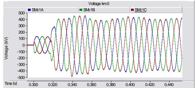
Fig. 14. Voltage at Serra da Mesa – km 0 – Simulation detail – 400 Ω pre-insertion resistor
