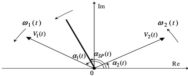
Fig. 17. A space synchrophasor is changing in a forward-forward mode.
