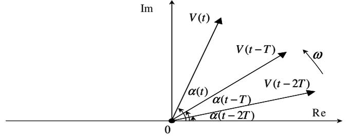
Fig. 13. A phasor is rotating in a forward mode.
