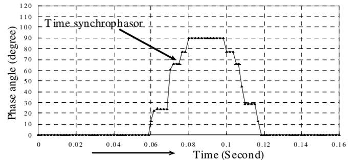
Fig. 30. Time synchrophasor in the phase step test (90°).
