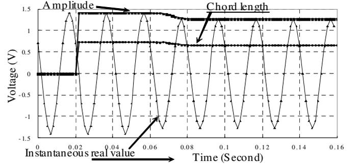
Fig. 27. Voltage instantaneous real values, measured amplitude and chord length in the magnitude step test (10%).
