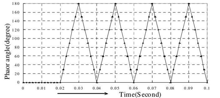
Fig. 11. Measured phasor with the proposed method (Case1).
