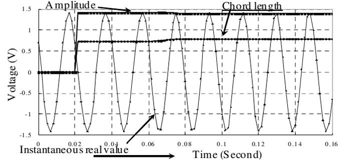
Fig. 31. Voltage instantaneous real values, measured amplitude and chord length in the frequency step test (+5Hz).
