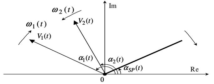
Fig. 20. A space synchrophasor is changing in a backward-forward mode.
