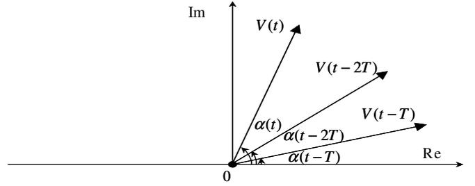
Fig. 15. A phasor is rotating in an inversion mode.
