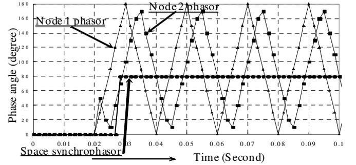
Fig. 24. Measured phasors and space synchrophasor with the proposed method (Case4).
