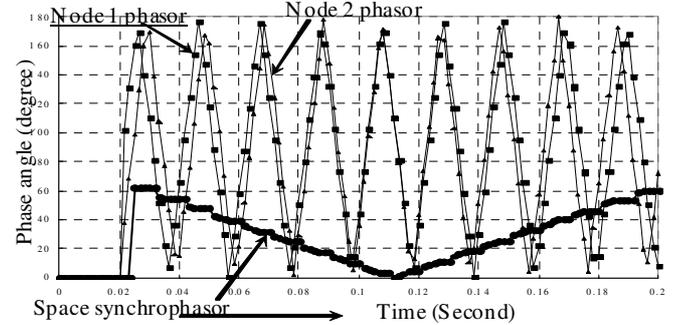
Fig.25. Measured phasors and space synchrophasor with the proposed method (Case5).
