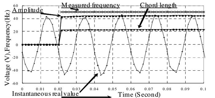
Fig. 34. Voltage instantaneous real values, measured amplitude and chord length in Case 7. (A harmonic distortions example)
