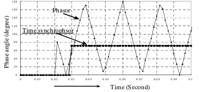
Fig. 23. Measured phasor and time synchrophasor with the proposed method (Case2).
