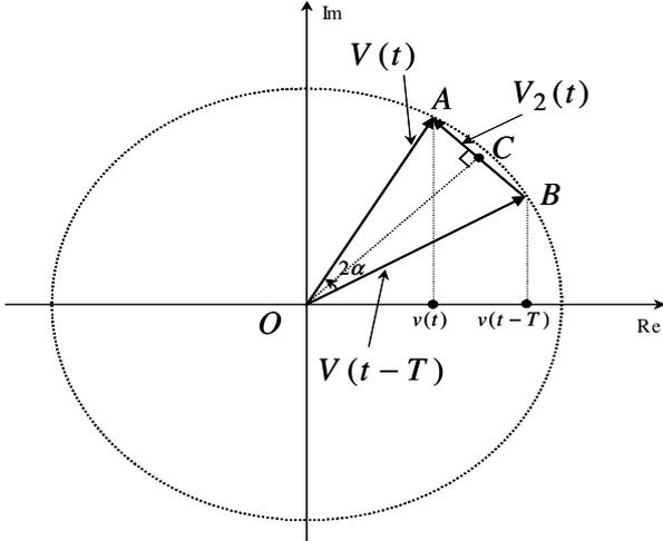
Fig. 2. A voltage spiral vector is rotating in one pitch period in the complex plane.
