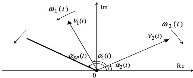
Fig. 19. A space synchrophasor is changing in a forward-backward mode.
