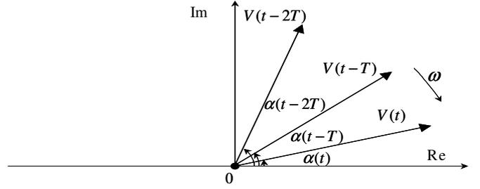
Fig. 14. A phasor is rotating in a backward mode.
