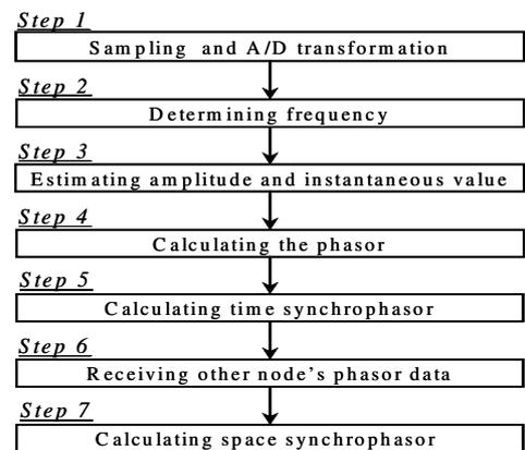
Fig. 22. The procedure for measuring synchrophasors.
