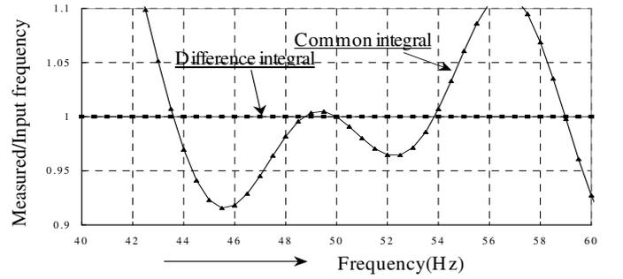
Fig. 9. Measured gain characteristics curves with common integral and difference integral method (Case2).
