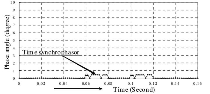
Fig. 28. Time synchrophasor in the magnitude step test (10%).
