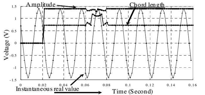
Fig. 29. Voltage instantaneous real values, measured amplitude and chord length in the phase step test (90°).
