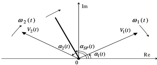
Fig.18. A space synchrophasor is changing in a backward-backward mode.
