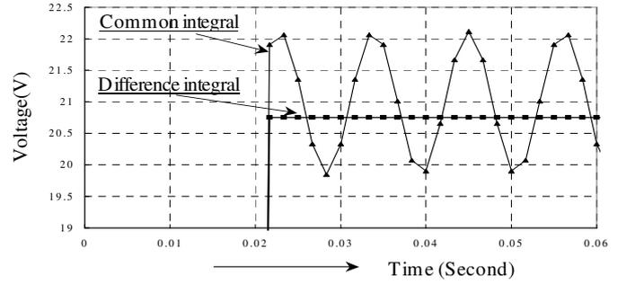
Fig. 5. Measured chord lengths with common integral method and difference integral method (Case2).
