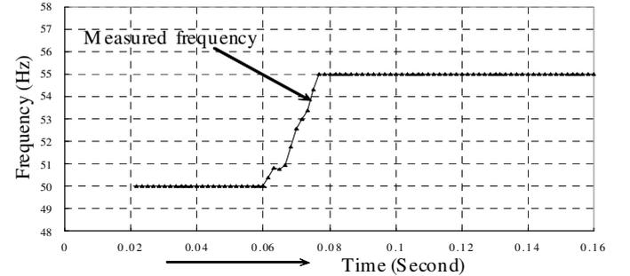
Fig. 33. Measured frequency in the frequency step test (+5Hz).
