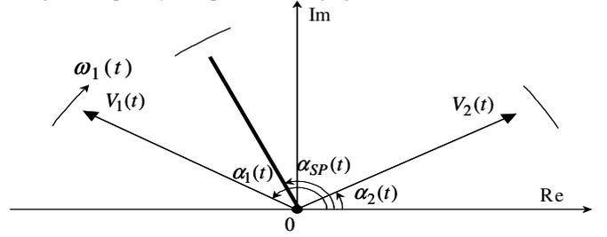
Fig. 21. A space synchrophasor is changing in a latch mode.
