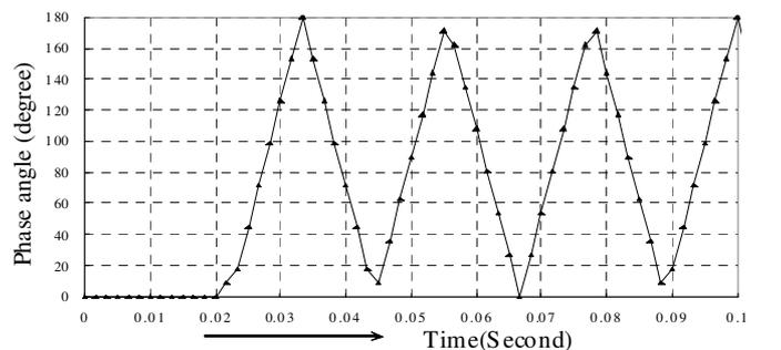
Fig. 12. Measured phasor with the proposed method (Case2).
