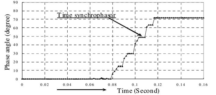
Fig. 32. Time synchrophasor in the frequency step test (+5Hz).
