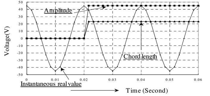
Fig. 3. Voltage instantaneous real values, measured amplitude and chord length with proposed integral method (Case1).
