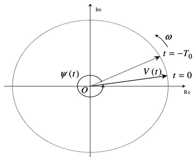
Fig. 1. A voltage spiral vector in the complex plane
