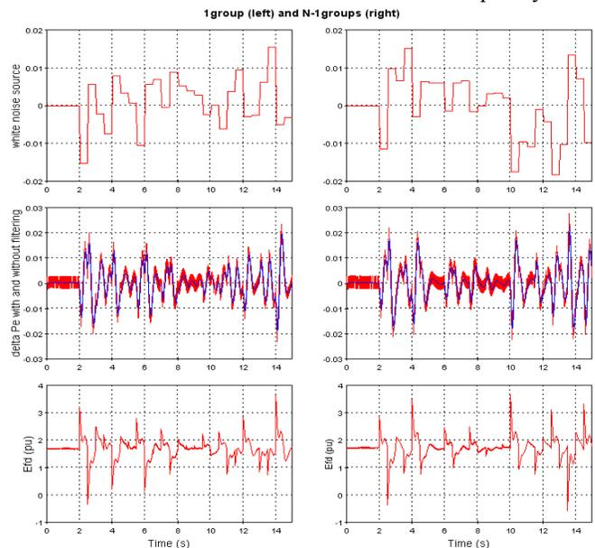
Fig. 3. Results from EMTPT time domain in open loop.
