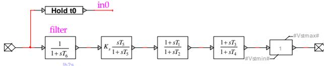
Fig. 4. IEEE PSS1A transfer function.  $P_e$  is filtered by the parameter  $T_6$
