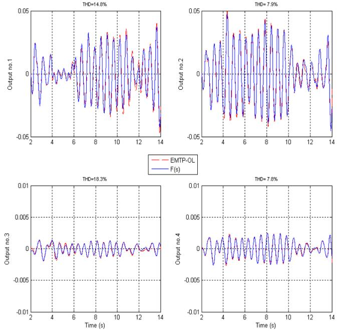
Fig. 6. Four outputs - Validation of  $F(s)$  with EMTP, PSS in open loop.
