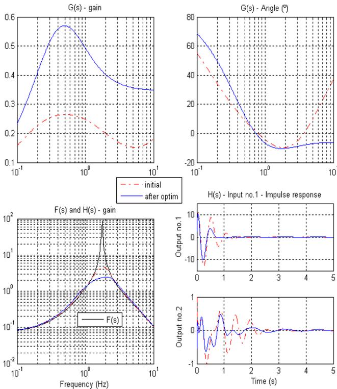
Fig.10. Bode diagram of F(s) and H(s). Time domain of H(s).
