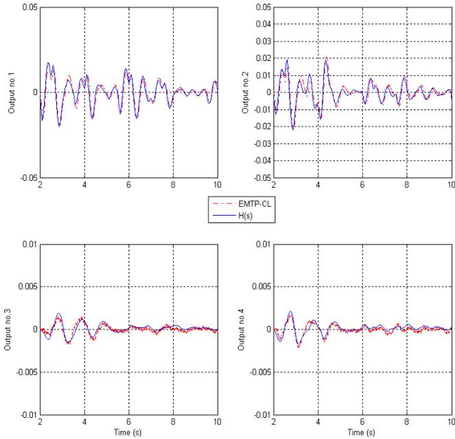
Fig.9 Harmonics included - Validation of  $H(s)$  with EMTP.
