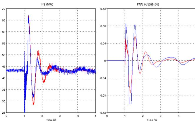
Fig. 13 Loss of line in EMTP. Initial (red) and after Optimization (blue).
