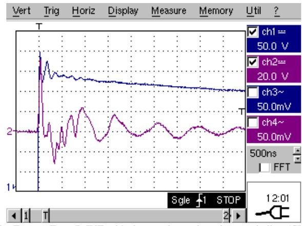
Fig. 8. Test on Type-B IVT with the supply on the primary winding (CH1) and open-circuit in both secondary windings (CH2 on the first secondary).
