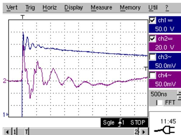
Fig. 9. Test on Type-B IVT with the supply on the primary winding (CH1) and open-circuit in both secondary windings (CH2 on the second secondary).
