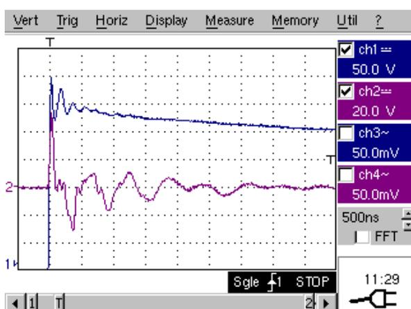
Fig. 11. Tests on Type-B IVT with the supply on the primary winding (CH1), short-circuit in the second secondary windings and open-circuit in the first secondary windings (CH2).
