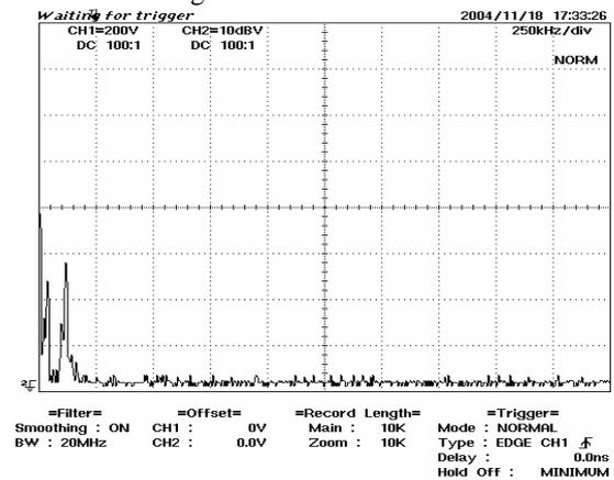
Fig. 1. DFT of the signal acquired at the IVT output when the primary circuit is fed by a very fast-front switching impulse.
