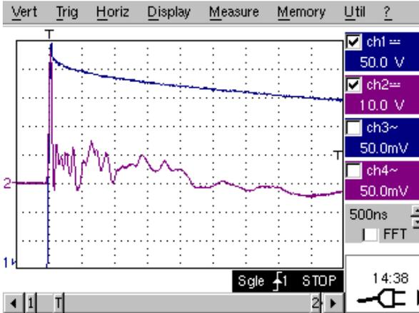
Fig. 5. Test on Type-A-2 IVT with the supply on the primary winding (CH1) and open-circuit in both secondary windings (CH2).
