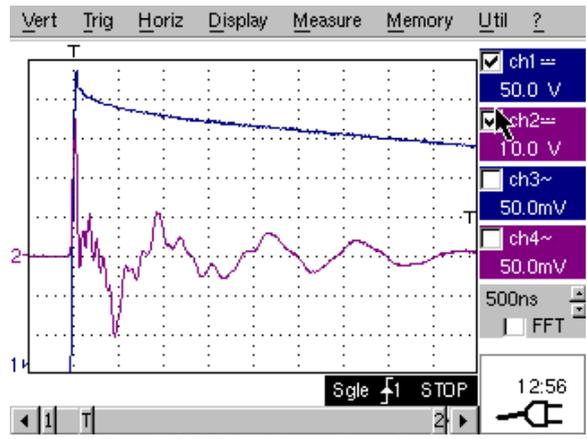
Fig. 7. Test on Type-A-2 IVT with the supply on the primary winding (CH1), short-circuit in one of the secondary windings and open-circuit in the other of the secondary windings (CH2).
