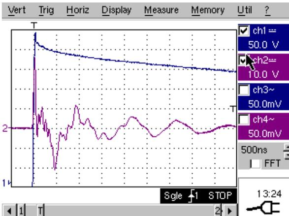
Fig. 6. Test on Type-A-1 IVT with the supply on the primary winding (CH1), short-circuit in one of the secondary windings and open-circuit in the other of the secondary windings (CH2).
