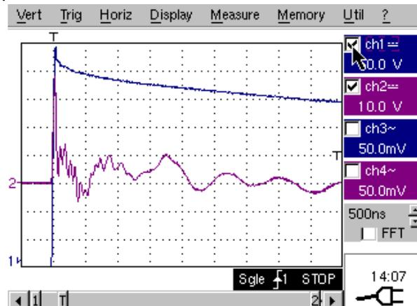
Fig. 4. Test on Type-A-1 IVT with the supply on the primary winding (CH1) and open-circuit in both secondary windings (CH2).
