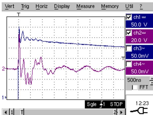
Fig. 10. Tests on Type-B IVT with the supply on the primary winding (CH1), short-circuit in the first secondary windings and open-circuit in the second secondary windings (CH2).
