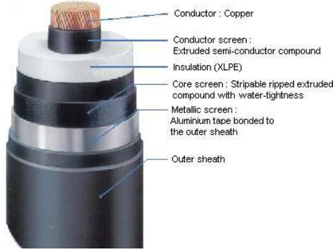
Fig. 7. Description of the different layers in the MV cable.
