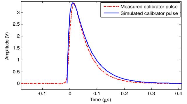
Fig. 7. Measured and simulated 5 nC calibrator pulses
