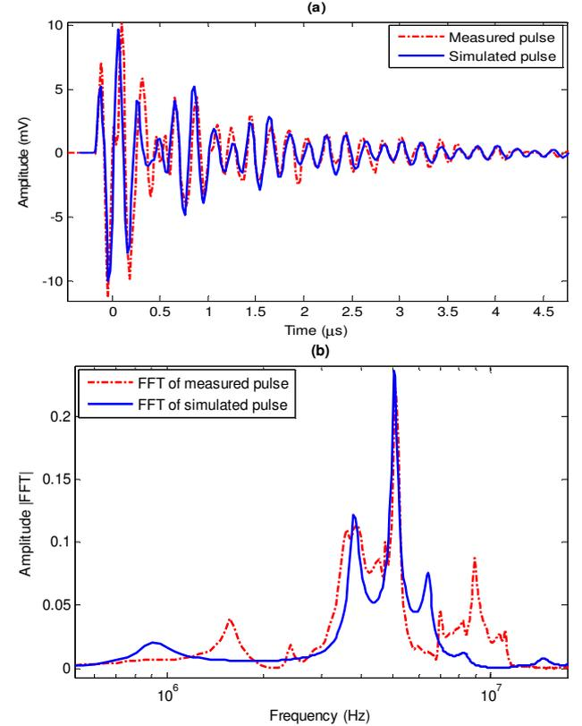
Fig. 8. The Rogowski coil response for 5 nC calibrator pulse at point P<sub>2</sub> in (a) time domain, and (b) frequency domain
