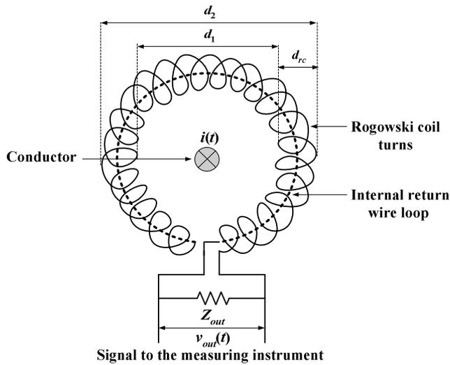
Fig. 1. Geometry and construction of the Rogowski coil.
