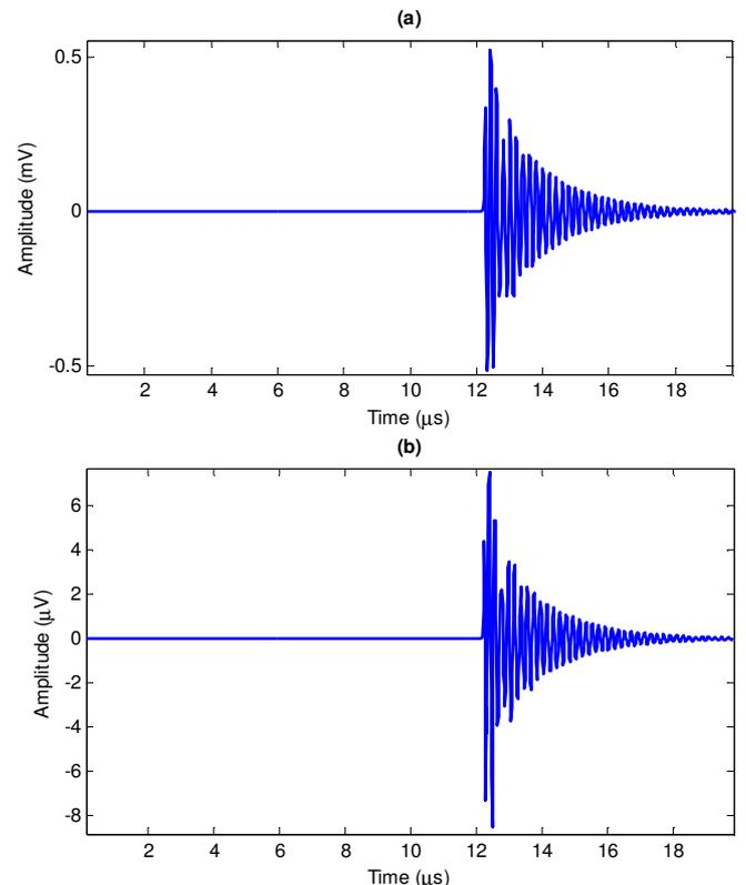
Fig. 10. Simulated Rogowski coil PD measurements due to leaning of a tree on phase A, keeping  $S_3=3.5$  km; (a) phase A, (b) phase B and C
