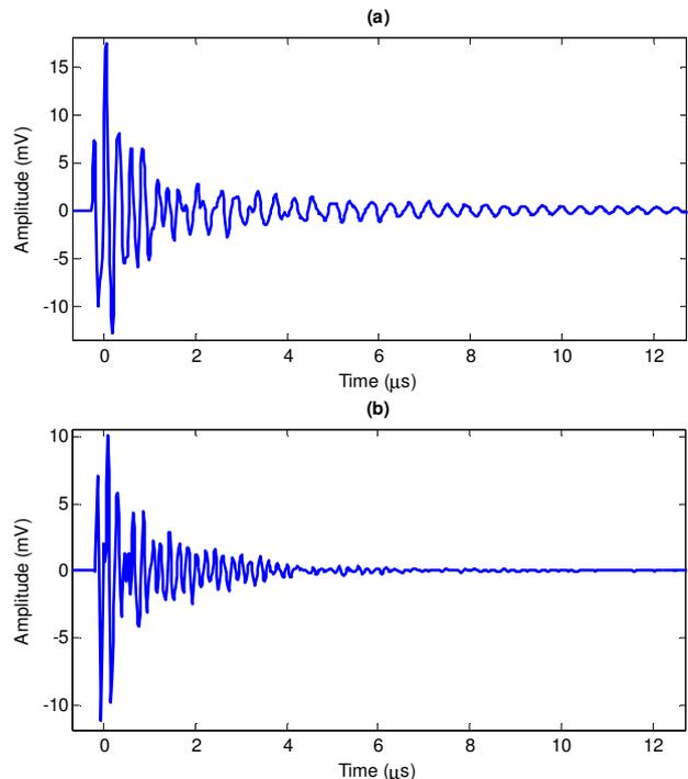
Fig. 5. Rogowski coil responses for 5 nC calibrator pulse at (a) point  $P_1$ , and (b) point  $P_2$
