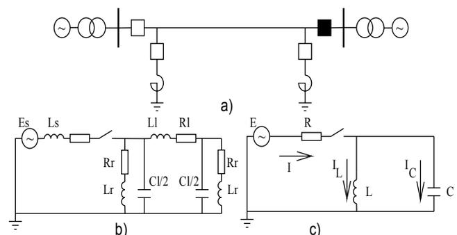
Fig. 1. Scheme of the transmission line under study and its equivalent circuits
