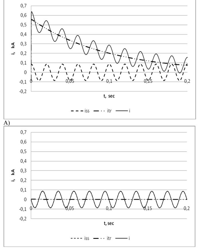
Fig. 2. Current through the circuit breaker A) if  $\psi = 0$  B) if  $\psi = \pi/2$ .
