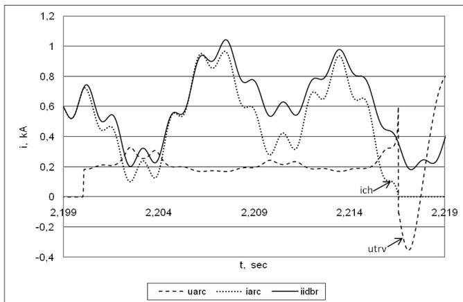
Fig. 3. Arc extinguishing process during air circuit breaker cutoff
