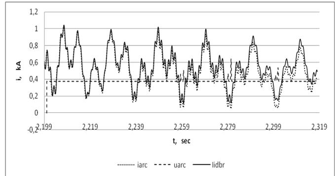
Fig. 4. Arc extinguishing process during SF6 circuit breaker cutoff
