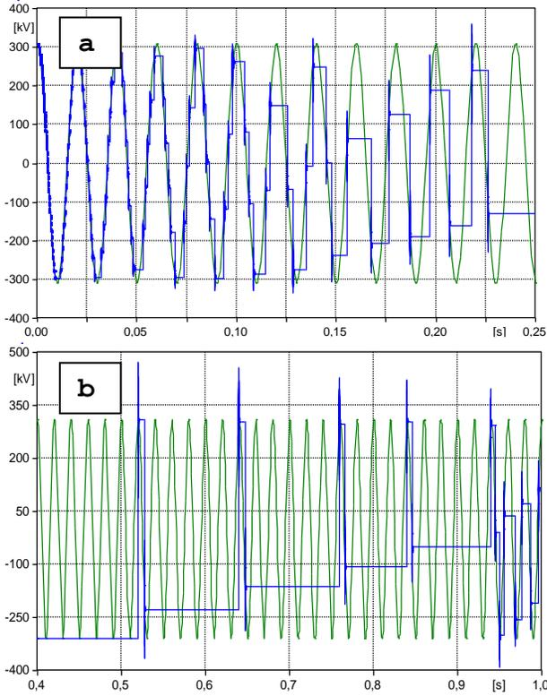
Fig. 5. VFT due to disconnector switching – source side voltage (continuously alternating) and load side voltage (step wise) for: a) **opening** (restrikes), b) **closing** (prestrikes) operation at disconnector terminals
