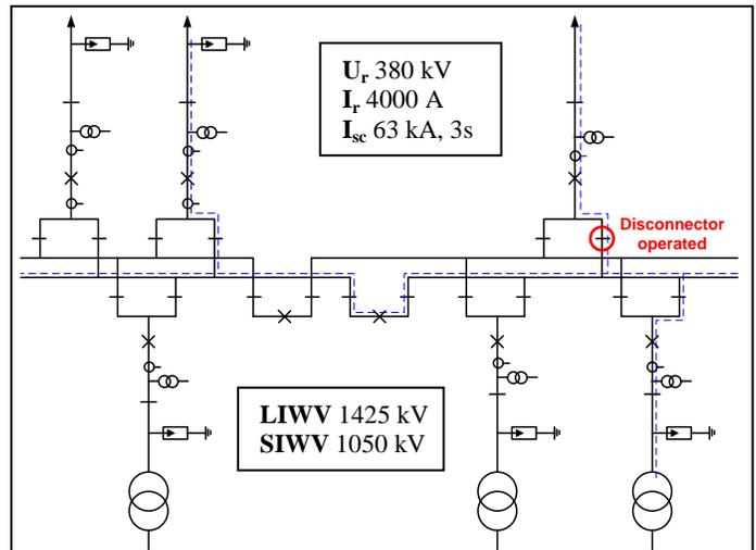
Fig. 4. Single line diagram of HV GIS substation with calculated configuration marked with the dashed line
