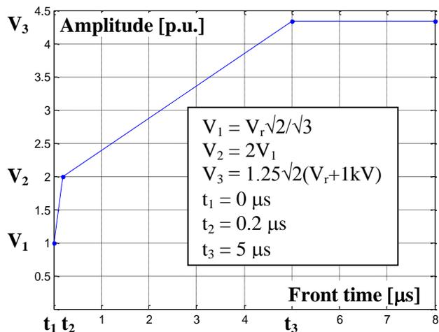
Fig. 1. Machine impulse withstand envelope [4]
