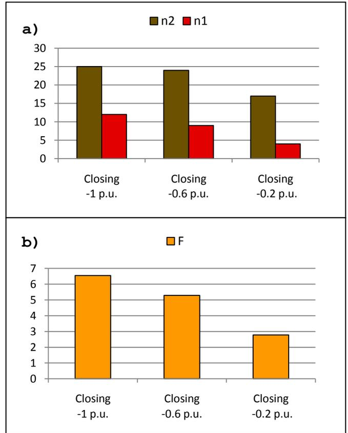
Fig. 7. a) Number  $n_1$  of VFT overvoltage exceeding withstand envelope (red coloured) and number  $n_2$  of VFT overvoltage exceeding 1 p.u. only (black coloured), b) value of the VFT quantitative measure, functional  $F$
