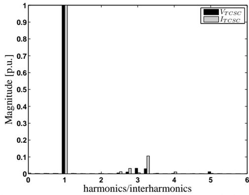
Fig. 7. Frequency content of the voltage at TCSC's terminals and of the current entering the TCSC.
