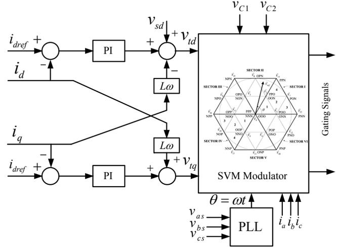
Fig. 7. Currents control block diagram
