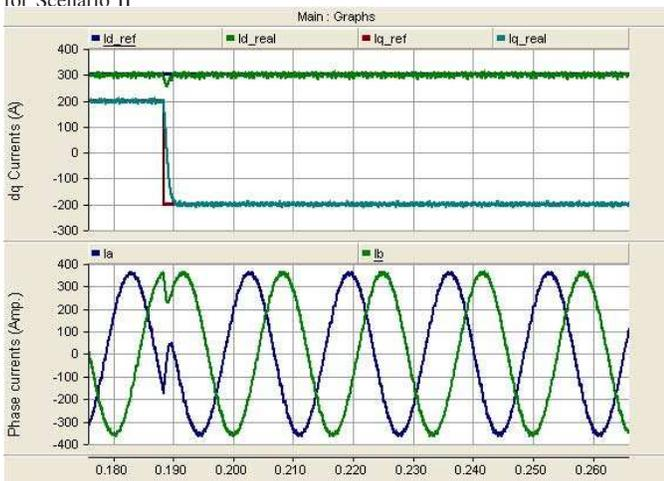
Fig. 12. The simulation results generated by the PSCAD/EMTDC for Scenario II
