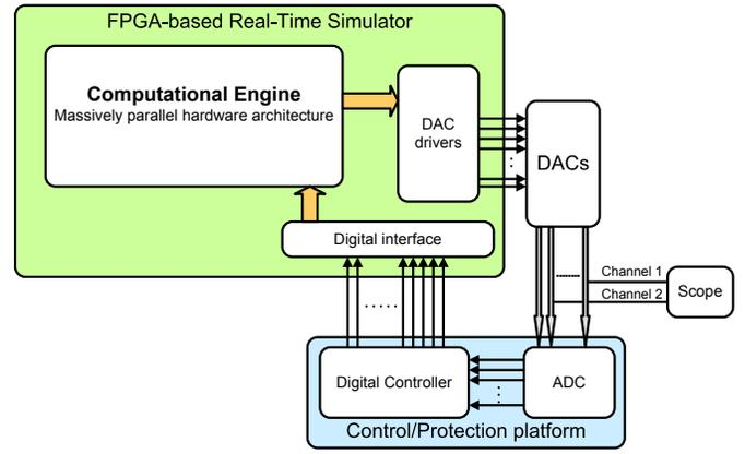
Fig. 2. Schematic of the FPGA-based real-time simulator in HIL testing arrangement
