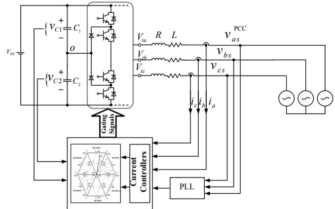
Fig. 6. Schematic diagram of the NPC converter system and its controller
