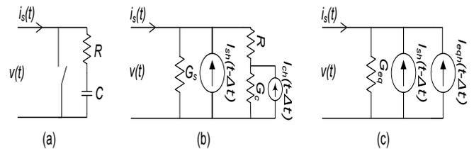
Fig. 3. (a) Switch with a snubber circuit (b) equivalent ADC model (c) Combined switch model
