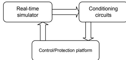
Fig. 1. HIL arrangement for closed-loop testing of controller platforms
