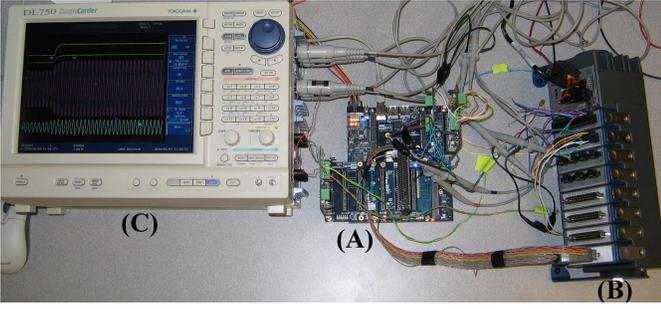
Fig. 8. Photo of the experimental setup: (A) the FPGA-based real-time simulator, (B) the CRIO controller platform, and (C) the oscilloscope
