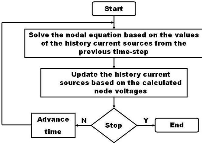
Fig. 4. Flowchart of the simulation process based on the adopted solution algorithm)
