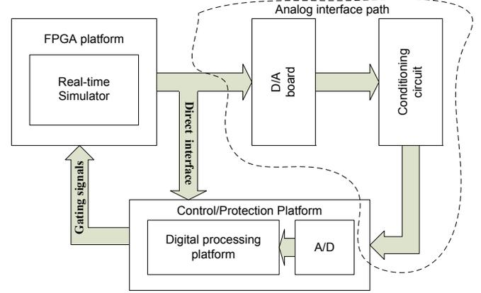
Fig. 5. Simulator/controller interface options
