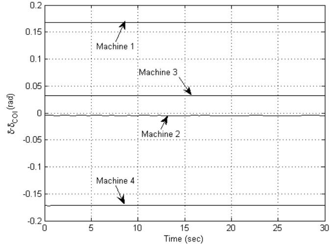
Fig. 7. The response of the system at steady state with the STATCOM
