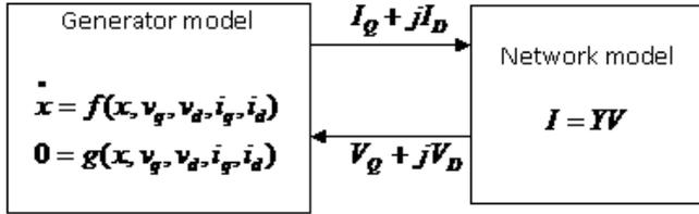
Fig. 1. Schematic diagram of the system
