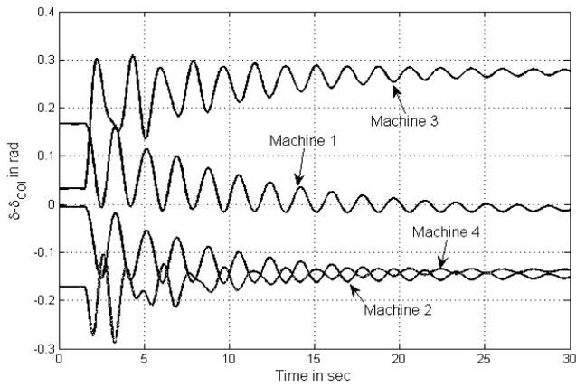
Fig. 9. The response of the system for a fault in line 7-8 with STATCOM
