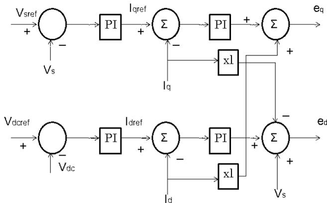
Fig. 3. Block diagram of Type I control strategy of STATCOM.
