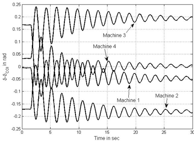
Fig. 15. The response of the system for a fault in line 10-8 with STATCOM
