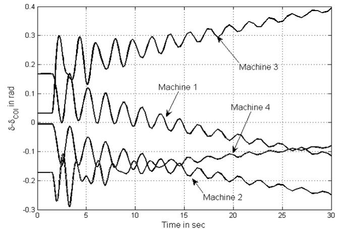
Fig. 8. The response of the system for a fault in line 7-8 without STATCOM
