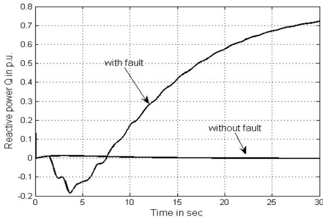
Fig. 10. STATCOM injected reactive power into the system
