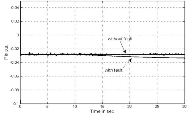
Fig. 12. STATCOM real power exchange to the system
