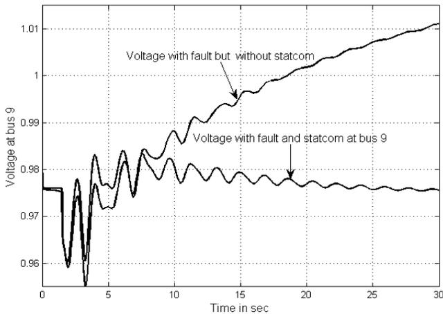
Fig. 11. Voltage at bus 9 of the system
