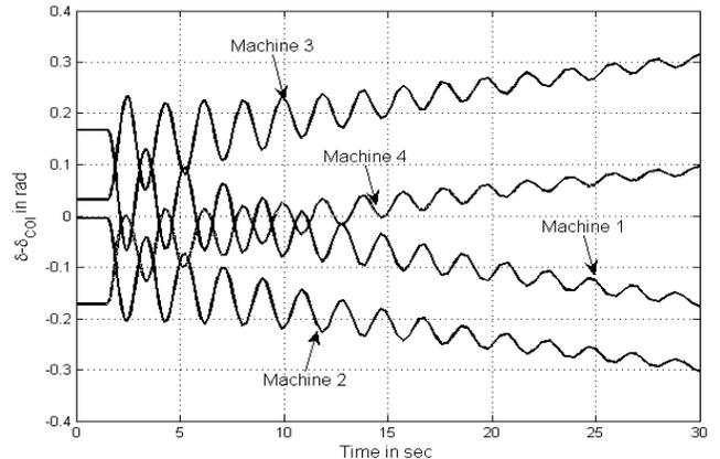
Fig. 14. The response of the system for a fault in line 10-8 without STATCOM
