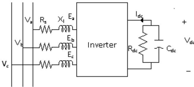
Fig. 2. Equivalent circuit of STATCOM.
