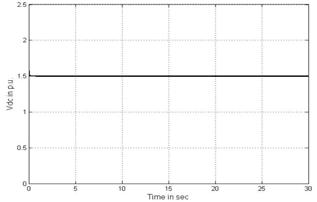
Fig. 13. STATCOM dc capacitor voltage
