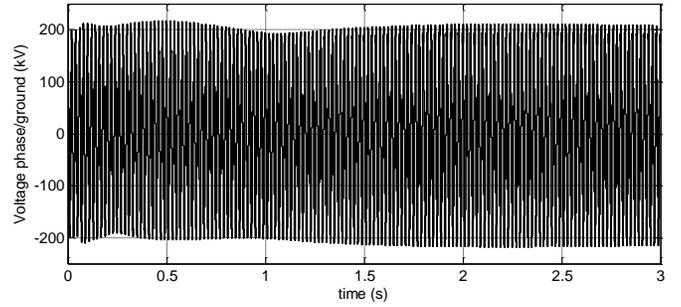
Fig. 7. Transformer energization at substation A. Voltage in phase A with complete network modeling
