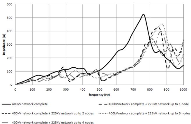
Fig. 2. Frequency responses of the network at Sub A for different sizes of 225 kV network modeling.
