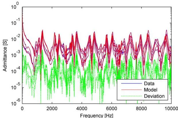
Fig. 4. Comparison between original frequency scan and FDNE at Sub A.
