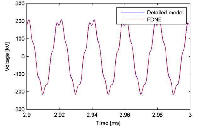
Fig. 9. Transformer energization at substation A, voltage phase A with complete network modeling and with FDNE, zoom on the last 100 ms.
