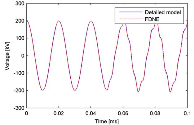
Fig. 8. Transformer energization at substation A, voltage phase A with complete network modeling and with FDNE, zoom on the first 100ms.
