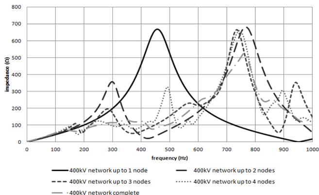
Fig. 1. Frequency responses of the network at Sub A for different sizes of 400 kV network modeling.
