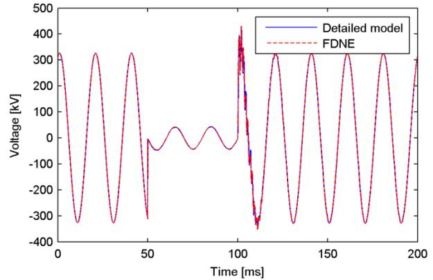
Fig. 5. Three-phase fault and clearing at the busbar of substation A, voltage in phase A with complete network modeling and with FDNE
