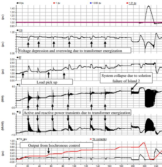
Fig. 3 Step-by-step Energization of the Island 1 with black start Generators loaded to 70 % of rated Capacity with modeling of Transformer Remanence
