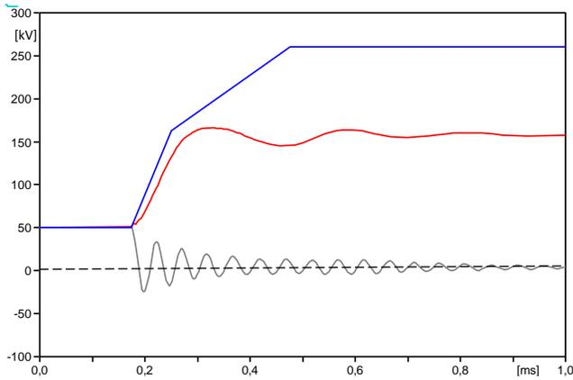
Fig. 6: Short line fault (75% - CB1) – Network configuration 3 (max short-circuit current).
