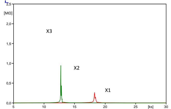
Fig. 9: frequency scan for three different series reactors connected.
