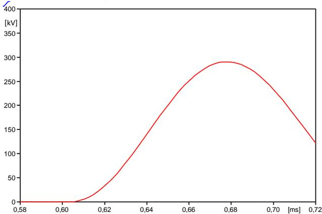
Fig. 8: CB1 TRV - fault at X3 reactor terminals – Network configuration III (max short-circuit current).
