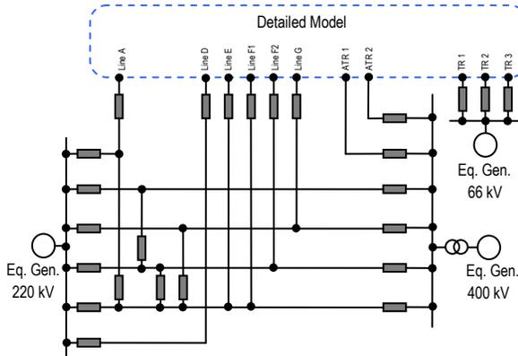
Fig. 3. Short circuit equivalent network model connected to the external boundary of the detailed model
