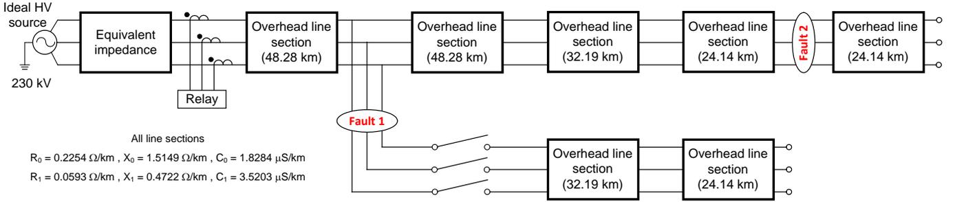
a) Transmission test system – 230 kV
