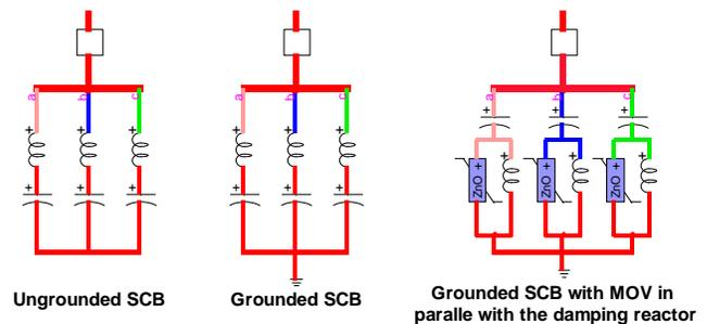
Fig. 1 Configurations of shunt capacitor banks under study
