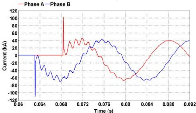
Fig.10 Current observed on phase A and B after a multi-phase reignition with a damping reactor of 3,5 mH
