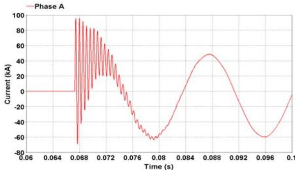
Fig.7 Current observed on the faulted phase after a reignition
