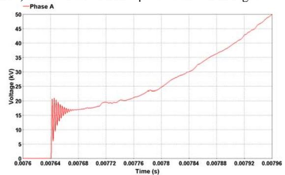
Fig.5 Front wave created by the damping reactor
