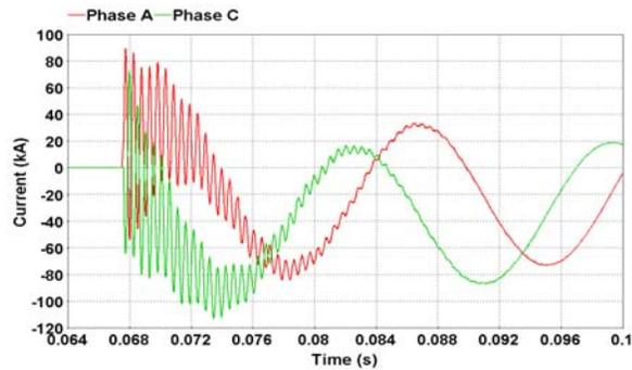
Fig.3 Current observed on phase A and C after a multi-phase reignition
