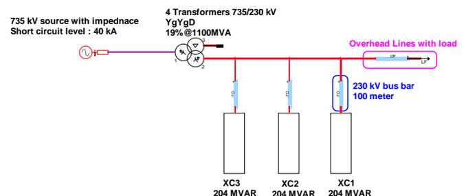
Fig. 2 EMTP-RV equivalent circuit of a 230 kV substation equipped with 3 shunt capacitor banks
