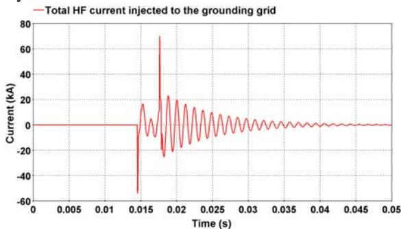
Fig.13 Total HF current injected to the grounding grid in case of three phase to ground fault
