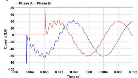
Fig.12 Current observed on phase A and B after a multi-phase reignition with a realistic representation of bus bar impedance between shunt capacitor banks
