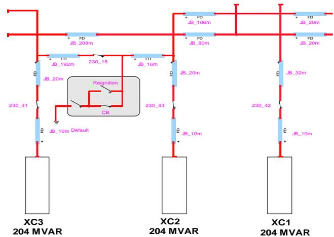
Fig.11b) A realistic representation of bus bar impedance between SCB
