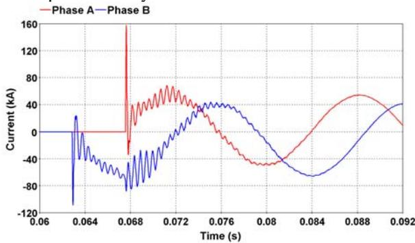
Fig.9 Current observed on phase A and B after a multi-phase reignition
