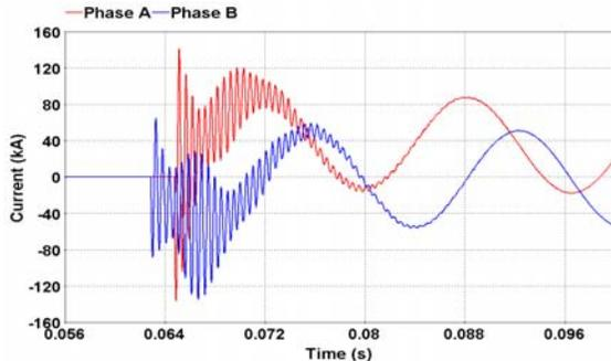
Fig.6 Current observed on phase A and C after a multi-phase reignition
