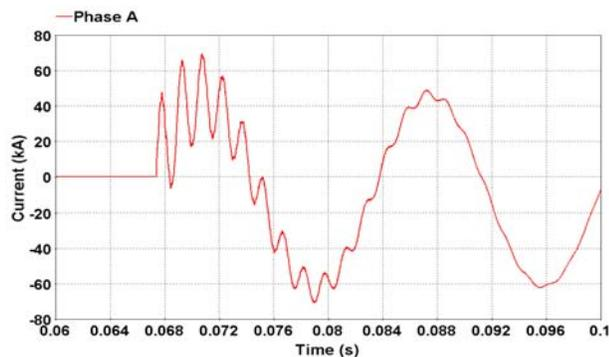
Fig.4 Current observed on the faulted phase after a reignition
