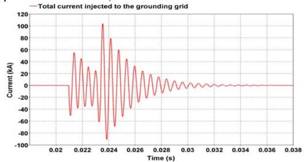
Fig.8 Total HF current injected to the grounding grid in case of three phase to ground fault
