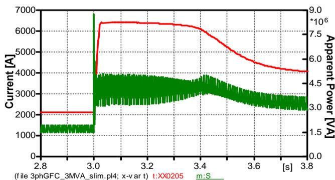
Fig. 21. GFC Output RMS Current & Apparent Power
