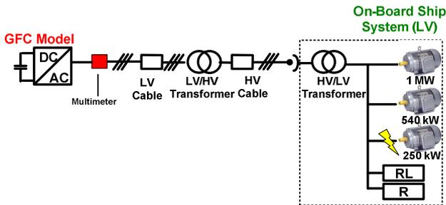
Fig. 16. Short-Circuit System
