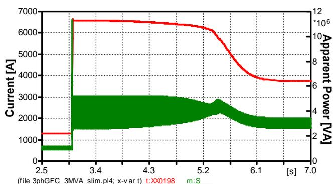
Fig. 20. GFC Output RMS Current & Apparent Power
