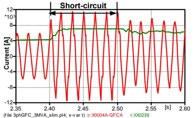
Fig. 19. GFC output current
