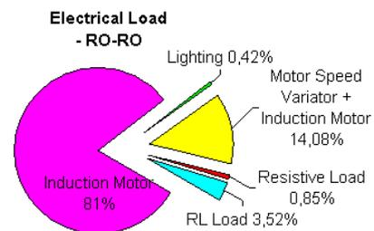
Fig. 2. RO-RO (Roll-on/roll-off ship – used to carry wheeled cargo) Load Breakdown
