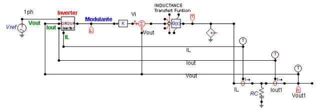
Fig. 5. Single-phase Inverter model in ATP-EMTP
