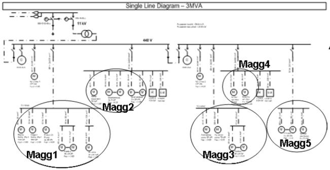
Fig. 6. Ship electrical system
