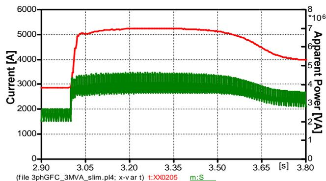
Fig. 22. GFC Output RMS Current & Apparent Power
