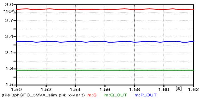
Fig. 14. GFC output power: red - Apparent Power [VA]; blue - Active Power [W]; green- Reactive Power [VAr]
