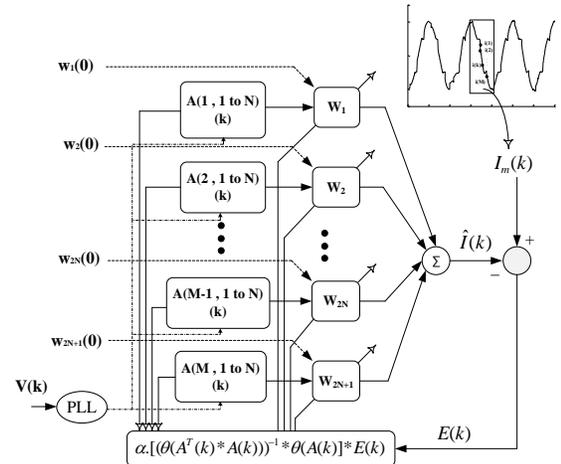
Fig. 6. Block diagram of the proposed W-Adaline algorithm
