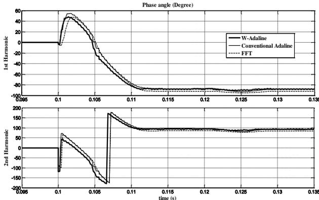
Fig. 16. Estimation of the phase angle of inrush current (1<sup>st</sup> and 2<sup>nd</sup> order harmonic)
