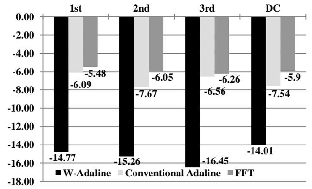
Fig. 12. Relative error of W-Adaline and conventional Adaline in estimating the amplitude
