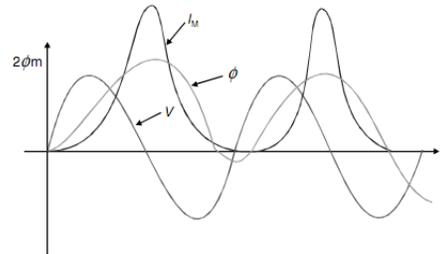
Fig. 3. Inrush current of a transformer
