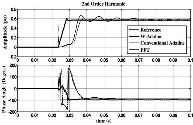
Fig. 9. Estimation of amplitude and phase angle of 2<sup>nd</sup> order harmonic
