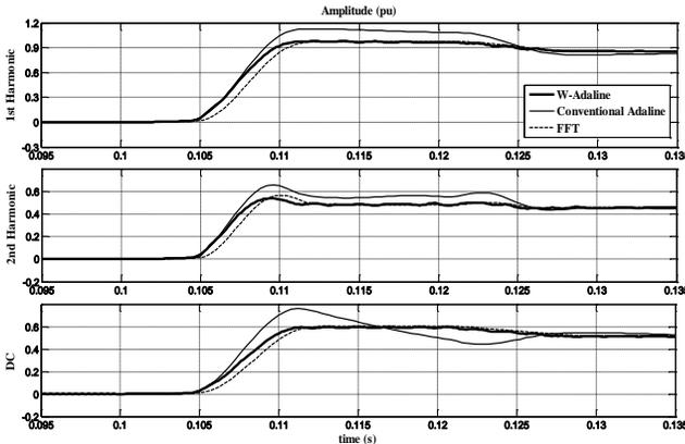
Fig. 15. Estimation of the amplitude of inrush current (1<sup>st</sup> and 2<sup>nd</sup> order harmonic and DC component)
