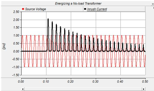
Fig. 14. Source voltage and inrush current of a case-study transformer
