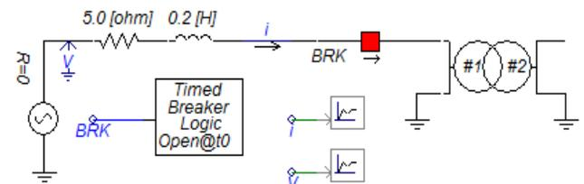
Fig. 13. Single line diagram of an energized transformer
