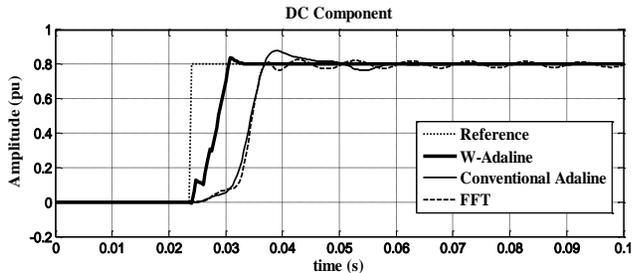
Fig. 11. Estimation of DC component
