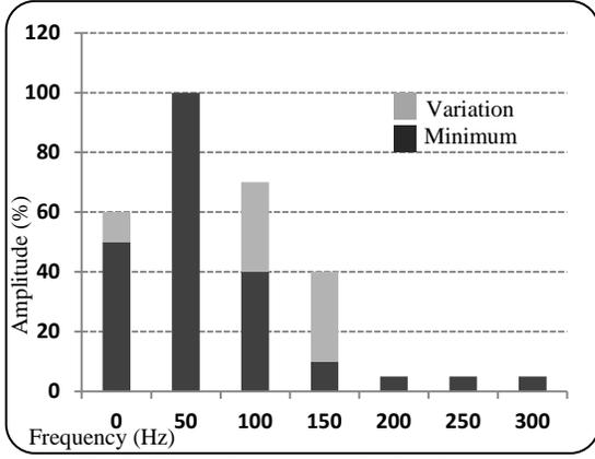
Fig. 4. Harmonic spectrum of an inrush current
