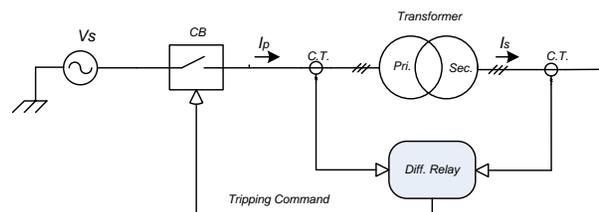
Fig. 1. Differential protection in a transformer
