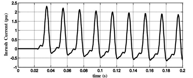
Fig. 7. Case-study signal of an inrush current
