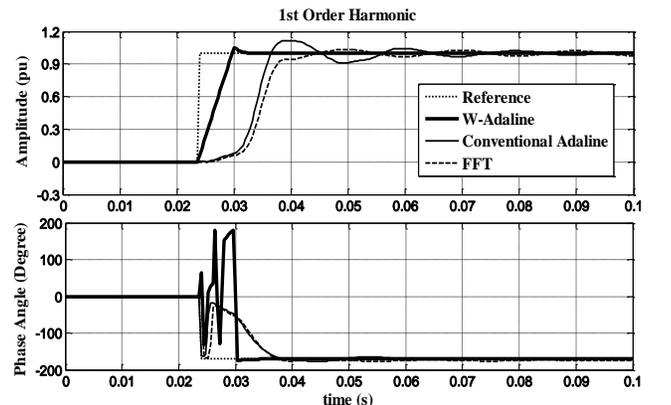
Fig. 8. Estimation of amplitude and phase angle of 1<sup>st</sup> order harmonic
