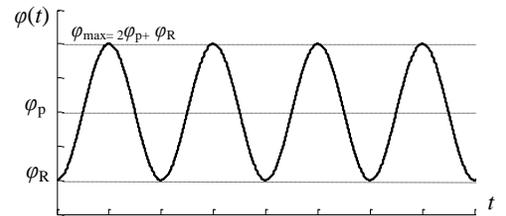
Fig. 2. Instantaneous flux of the transformer at the moment of energizing
