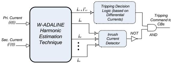
Fig. 5. Logical structure to identify the inrush current of a transformer
