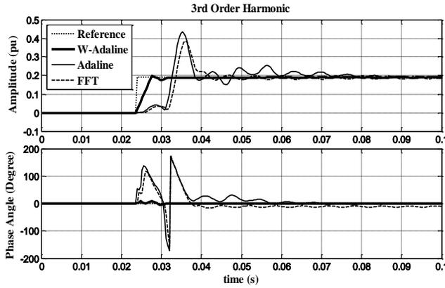
Fig. 10. Estimation of amplitude and phase angle of 3<sup>rd</sup> order harmonic
