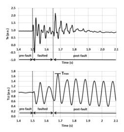
Fig. 9. Electrical torque and torque between masses of the two-mass shaft model for the case of a 150 ms fault at line between bus 4 and SC9
