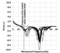
Fig. 8. Subsynchronous damping of the system after the fault clearance in Case II
