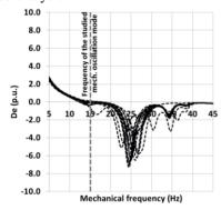
Fig. 7. Subsynchronous damping of the system after the fault clearance in Case I
