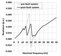
Fig. 4. Reactance curve for pre-fault and post-fault system conditions corresponding to an arbitrary fault and operating conditions of the system
