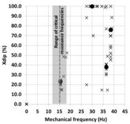
Fig. 6. Reactance dips for pre-fault and post-fault system conditions detected for Case II
