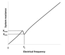
Fig. 1. Detection of the electrical system resonance frequencies
