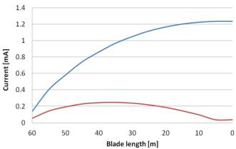
Fig.12. Maximum value of current induced in the wire for case 1: wire connected at the root (blue trace) and Case 2: wire floating (red trace). blade. Current impulse corresponding to the subsequent return stroke.
