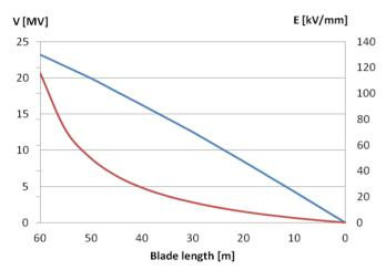
Fig.15. Maximum voltage difference V[MV] between the lightning conductor and the wire (blue trace) and average electric field E [kV/mm] (red trace) for case 1. Current impulse corresponding to the subsequent return stroke.
