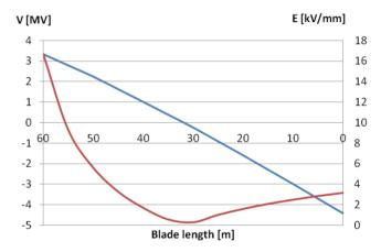
Fig.17. Maximum voltage difference V[MV] between the lightning conductor and the wire (blue trace) and average electric field E [kV/mm] (red trace) for case 2. Current impulse corresponding to the first return stroke negative.
