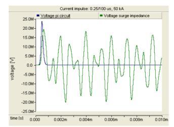
Fig.8. Model 1: Voltage drop across the lighting down conductor of the blade for the  $\pi$ -lumped circuit (blue trace) and the transmission line (green trace). Current impulse corresponding to the subsequent return stroke.
