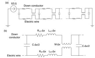
Fig.4. (a) Equivalent circuit of Model 2, (b) Single 5-meter section of Model 2, consisting of the resistance and inductance of the lightning conductor and internal electrical wire, and their inductive and capacitive coupling .
