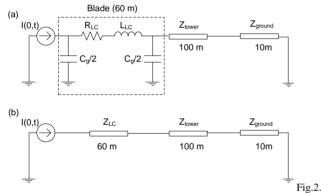
Equivalent circuit of the wind turbine, where the blade is modeled (a) as a  $\pi$ -lumped circuit and (b) as a transmission line.
