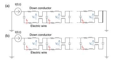
Fig.9. Model 2: Voltage and current measurements in (a) case 1, equipotential bonding between the wire and the down conductor at the root of the blade and (b) floating wire
