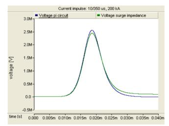
Fig.6. Model 1: Voltage drop across the lighting down conductor of the blade for the  $\pi$ -lumped circuit (blue trace) and the transmission line (green trace). Current impulse corresponding to the first return stroke positive.
