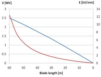
Fig.13. Maximum voltage difference V[MV] between the lightning conductor and the wire (blue trace) and average electric field E [kV/mm] (red trace) for case 1. Current impulse corresponding to the first return stroke positive.
