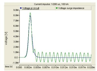
Fig.7. Model 1: Voltage drop across the lighting down conductor of the blade for the  $\pi$ -lumped circuit (blue trace) and the transmission line (green trace). Current impulse corresponding to the first return stroke negative.
