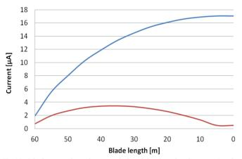
Fig.11. Maximum value of current induced in the wire for case 1: wire connected at the root (blue trace) and Case 2: wire floating (red trace). Current impulse corresponding to the first return stroke negative.
