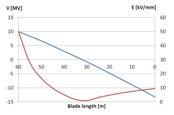
Fig.18. Maximum voltage difference V[MV] between the lightning conductor and the wire (blue trace) and average electric field E [kV/mm] (red trace) for case 2. Current impulse corresponding to the subsequent return stroke.
