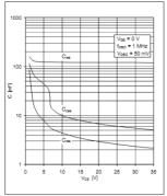
Figure 7: The non-linear capacitance-voltage characteristic of an IGBT [8]
