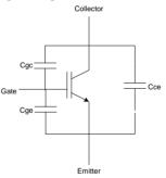
Figure 6: Capacitances of an IGBT [7]
