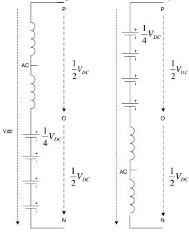
Figure 2: Operation of MMC single-phase diagram, on the right all lower submodule on and all upper submodule of. To the left the opposite case.
