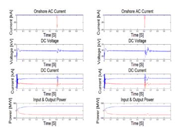
Figure 10: On the left *MMC response to dc link short circuit fault* a) AC phase voltage b) AC phase current c) DC link voltage for one pole d) DC current e) Active power transfer, on the right *MMC response to dc link short circuit fault* with increased transformer series capacitance.
