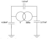
Figure 8: Implementation of transformer capacitances
