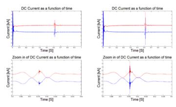
Figure 11: On the left MMC response to dc link short circuit fault a) DC current b) zoom in on the DC current. On the right MMC response to dc link short circuit fault with increased converter parasitic capacitance
