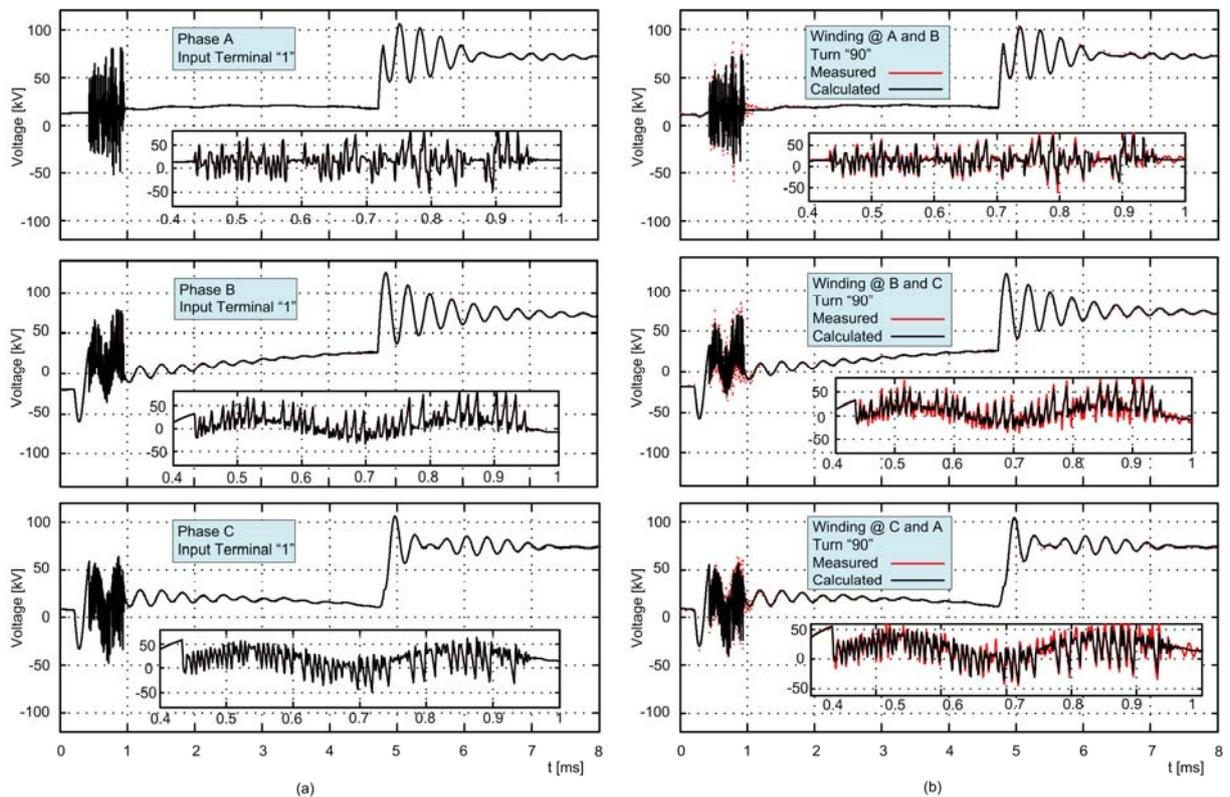
Fig. 5. Measured and computed voltages for opening operation of the VCB at the three windings at the phases A, B and C at: (a) terminals of the windings and (b) 90<sup>th</sup> turns in the windings.
