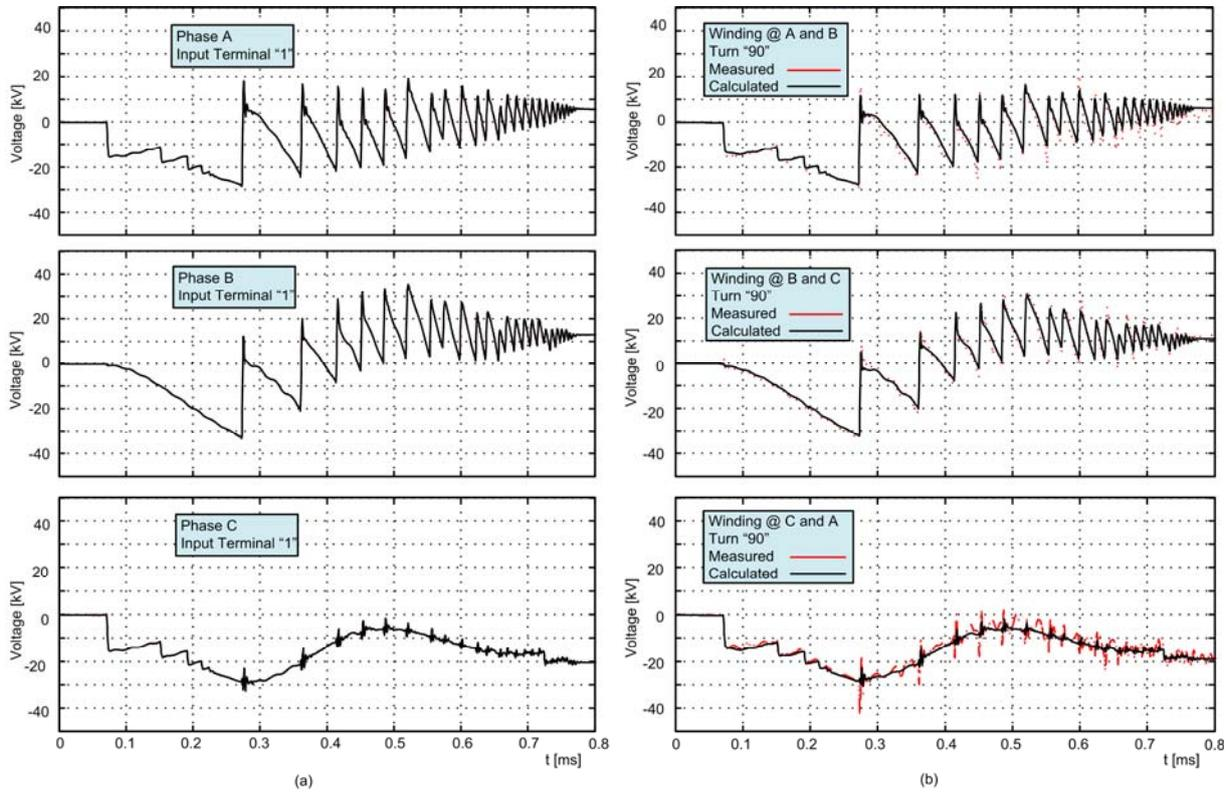
Fig. 4. Measured and computed voltages for closing operation of the VCB at the three windings at the phases A, B and C at: (a) terminals of the windings and (b) 90<sup>th</sup> turns in the windings.
