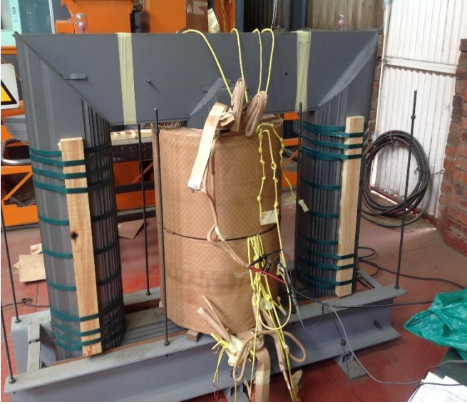
Fig. 4. Prototype transformer with measuring taps installed.
