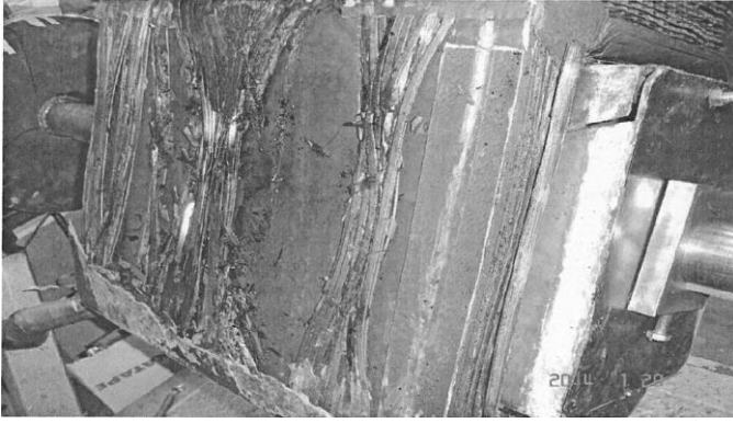
Fig. 1. Failed winding with inter-turn insulation severely damaged.
