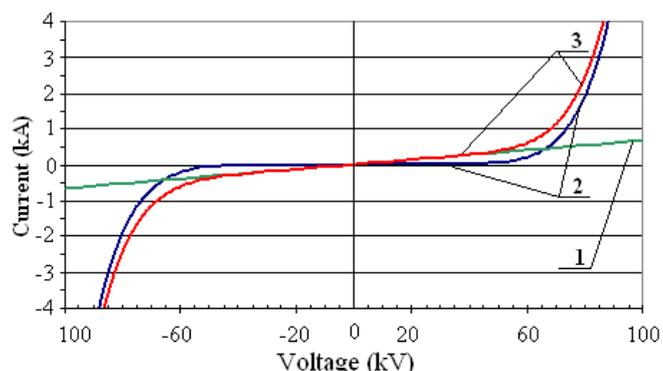
Fig. 1. Current-voltage characteristic of a limistor
