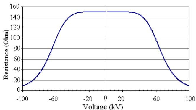
Fig. 2. Resistance versus voltage characteristic of a limistor
