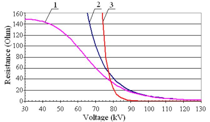
Fig. 7. Resistance of the limistor and surge arrester versus voltage characteristics (1 –  $R_{lim}$ , 2 –  $R_{nonlin}$ , 3 –  $R_{arrest}$ )
