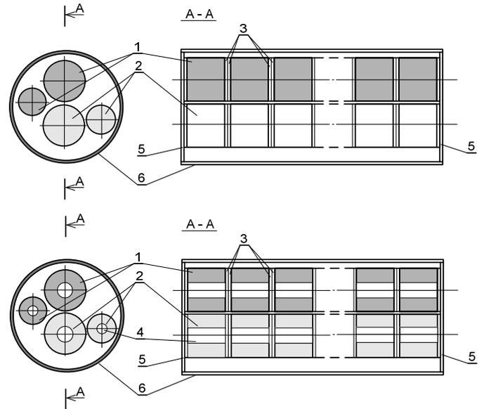
Fig. 3. Example of heterogeneous limistor, based on parallel connected  $N$  ( $N \geq 1$ ) linear and  $M$  ( $M \geq 1$ ) nonlinear resistors
