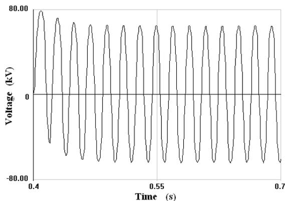
Fig. 6. Transient voltage at the grounded side of the shunt reactor with a limistor connected
