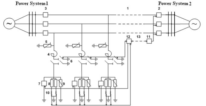
Fig. 4. Compensated transmission line with a resistor connected into the circuit of each shunt reactor
