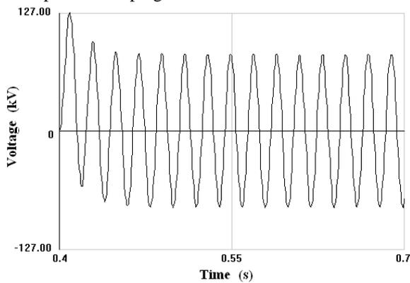
Fig. 5. Transient voltage at the grounded side of the shunt reactor with a linear resistor connected
