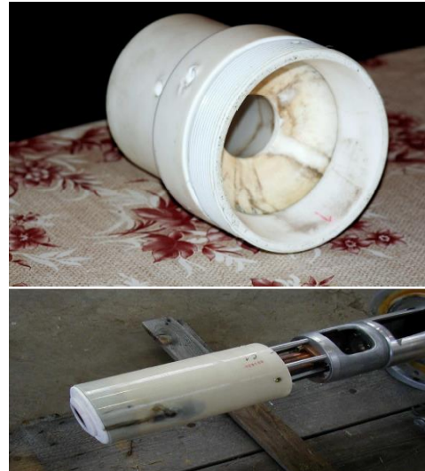
Fig. 2 Circuit breaker (parts of the contact systems after breakdown)
