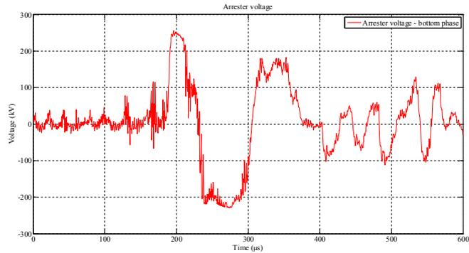
Fig. 7. Arrester voltage – case 1.
