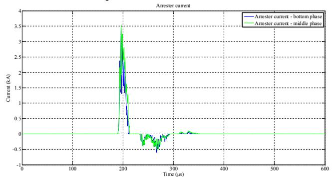
Fig. 11. Currents through arresters – case 2.
