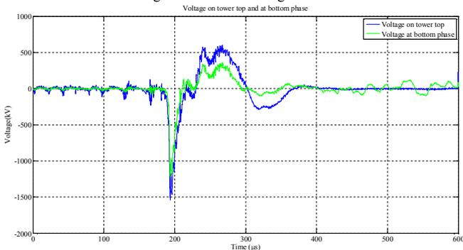
Fig. 15. Voltages on the tower top and at the bottom phase – case 2.
