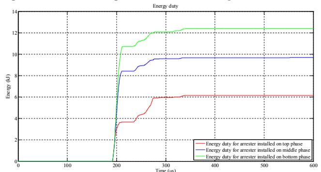
Fig. 18. Energy duties for arresters – case 3.
