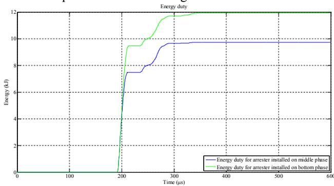
Fig. 13. Energy duties for arresters – case 2.
