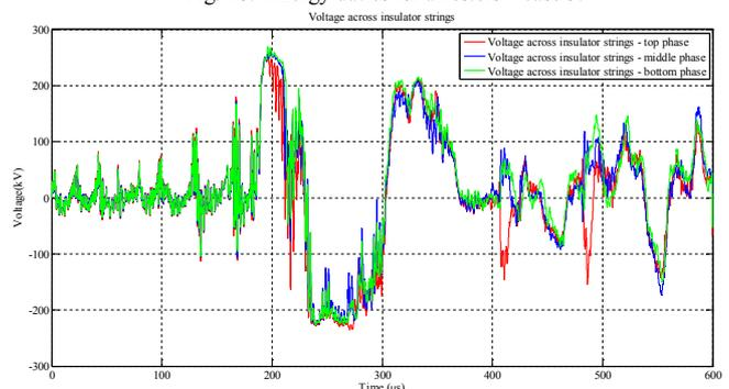
Fig. 19. Insulator voltages – case 3.
