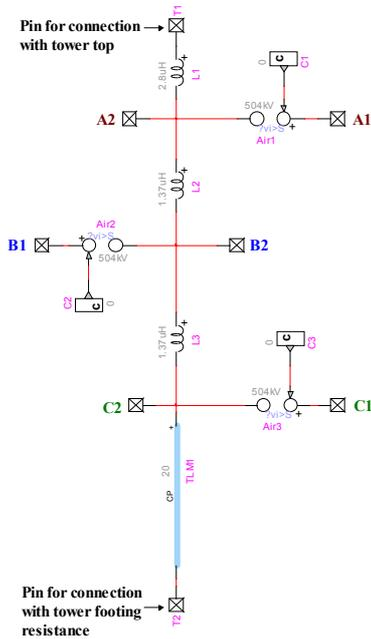
Fig. 2. Tower model in EMTP – RV.
