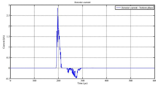
Fig. 6. Current through arrester – case 1.
