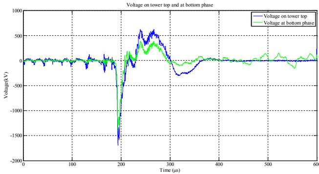
Fig. 20. Voltages on the tower top and at the bottom phase – case 3.
