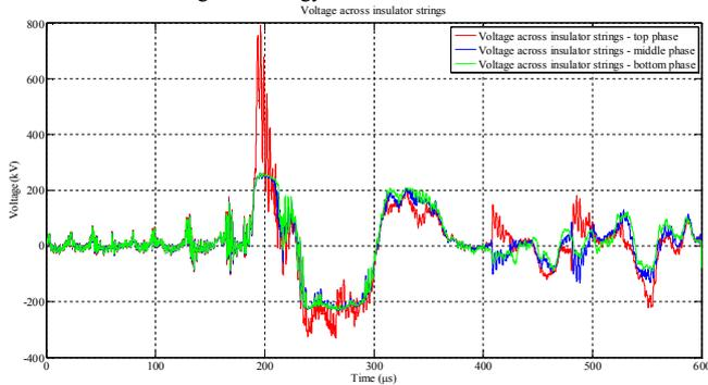
Fig. 14. Insulator voltages – case 2.
