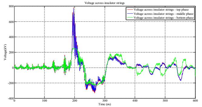
Fig. 9. Insulator voltages – case 1.
