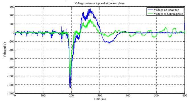
Fig. 10. Voltages on the tower top and at the bottom phase – case 1.
