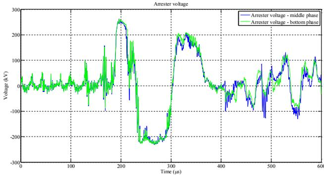
Fig. 12. Voltages on arresters – case 2.
