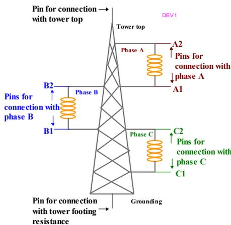
Fig. 3. EMTP – RV symbol for tower subcircuit.
