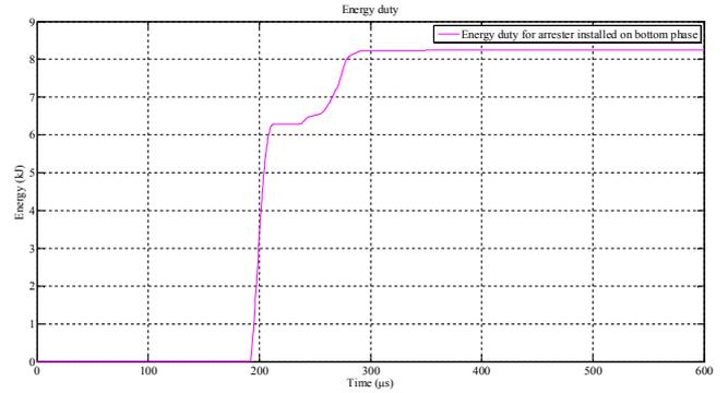
Fig. 8. Energy duty for arrester – case 1.
