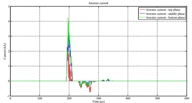
Fig. 16. Currents through arresters – case 3.
