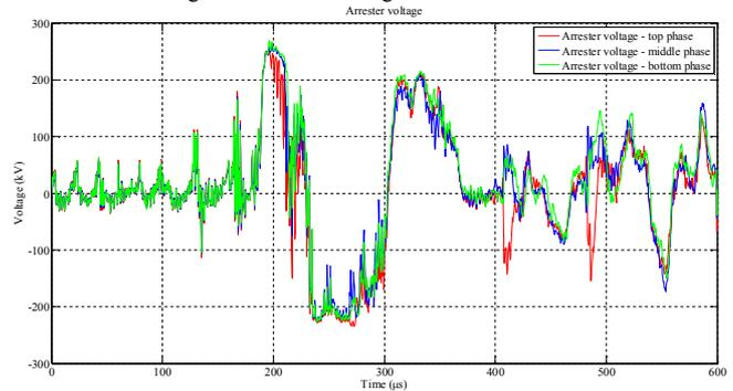
Fig. 17. Voltages on arresters – case 3.
