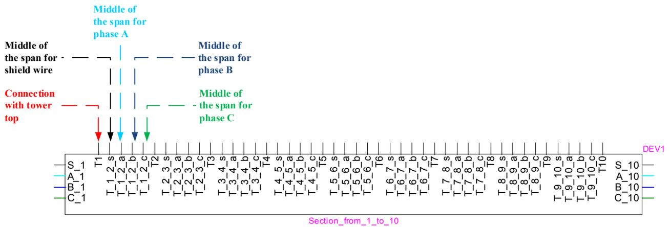
Fig. 5. EMTP – RV section of 110 kV transmission line.
