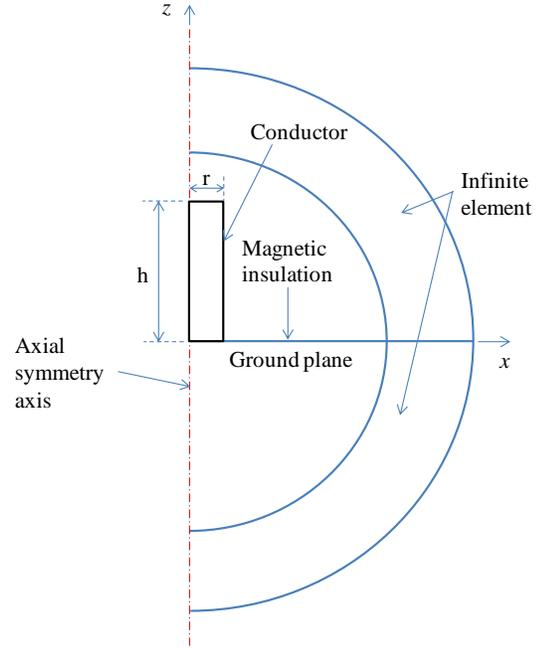
Fig. 1. Geometrical setup for FEM simulation
