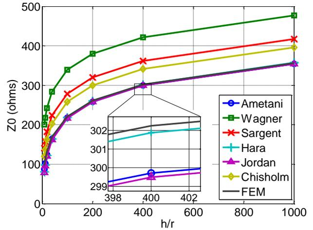
Fig. 2. Characteristic impedance of vertical conductor as a function of the  $h/r$  ratio
