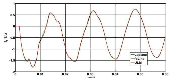
Fig. 26. Detail of current at shorted conductor 3 of delta line.
