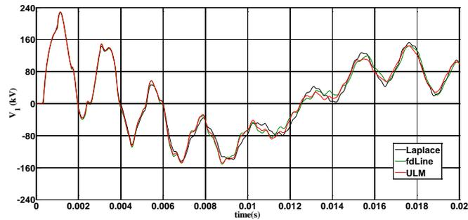
Fig. 30. Further detail of voltage at open conductor 1 of double-circuit one-tower delta line.
