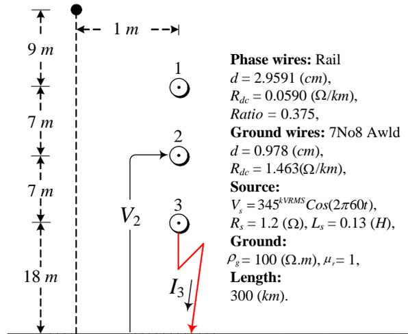
Fig. 3. Three-phase single-circuit vertical transmission line. ( $\Delta t = 50 \mu s$ )
