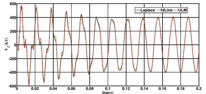
Fig. 16. Voltage at open conductor 2 of vertical line.
