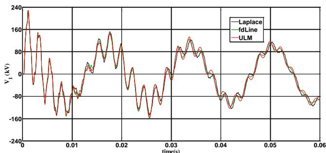
Fig. 29. Detail of voltage at open conductor 1 of double-circuit one-tower delta line.
