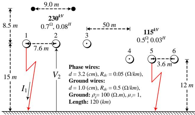
Fig. 6: Three-phase double-circuit two-tower horizontal transmission line. ( $\Delta t = 20 \mu s$ )
