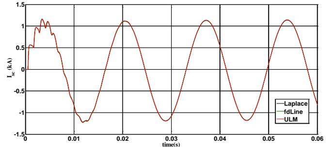
Fig. 9: Current at receiving-end of shorted single-phase line.
