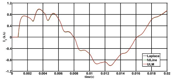
Fig. 15. Further detail of current at shorted conductor 1 of horizontal line.
