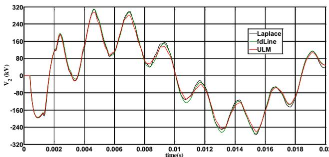
Fig. 36. Further detail of voltage at open conductor 2 of two parallel horizontal lines
