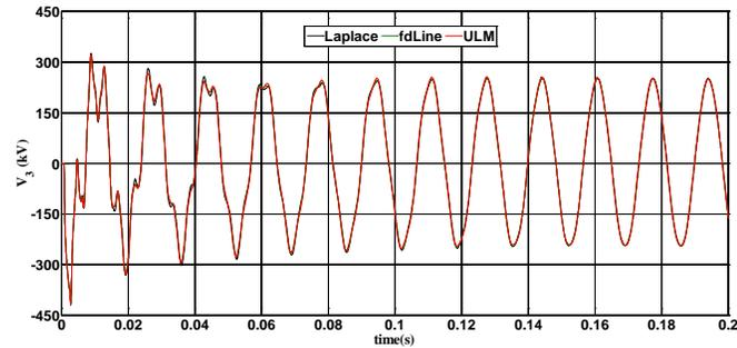
Fig. 10. Voltage at open conductor 3 of horizontal line.
