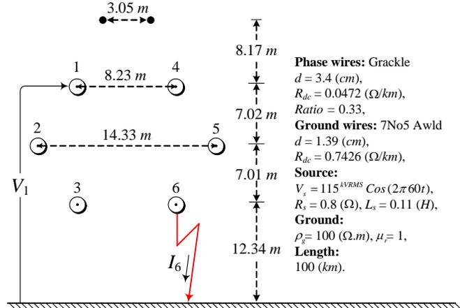
Fig. 5: Three-phase double-circuit one-tower delta transmission line. ( $\Delta t = 16 \mu s$ )
