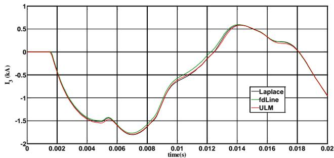
Fig. 27. Further detail of current at shorted conductor 3 of delta line.
