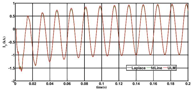
Fig. 19. Current at shorted conductor 3 of vertical line.
