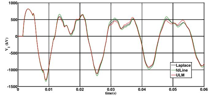
Fig. 23. Detail of voltage at open conductor 1 of delta line.
