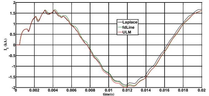
Fig. 39. Further detail of current at shorted conductor 1 of two parallel horizontal lines.
