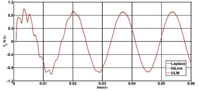
Fig. 14. Detail of current at shorted conductor 1 of horizontal line.
