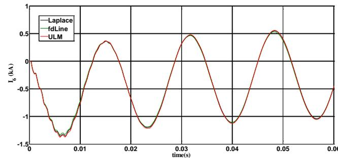
Fig. 32. Detail of current at shorted conductor 6 of double-circuit one-tower delta line.
