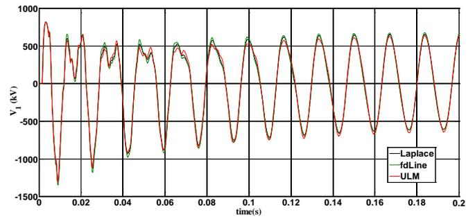
Fig. 22. Voltage at open conductor 1 of delta line.
