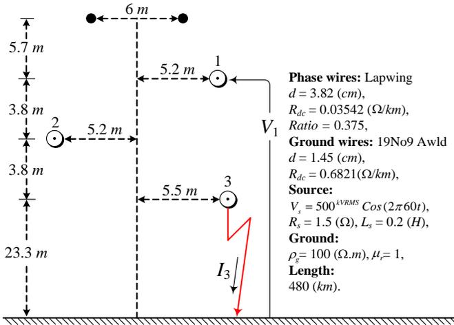
Fig. 4: Three-phase single-circuit delta transmission line. ( $\Delta t = 80 \mu s$ )
