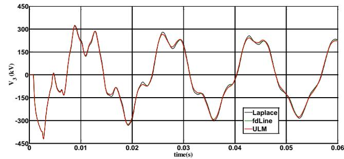
Fig. 11. Detail of voltage at open conductor 3 of horizontal line.
