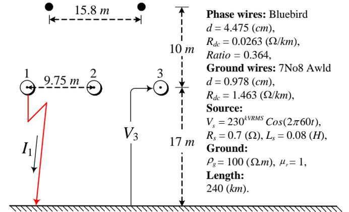
Fig. 2. Three-phase single-circuit horizontal transmission line. ( $\Delta t = 40 \mu s$ )
