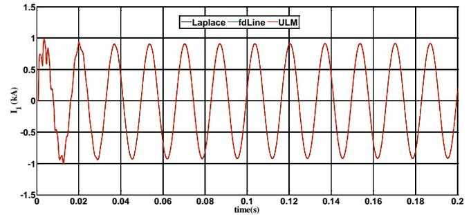
Fig. 13. Current at shorted conductor 1 of horizontal line.
