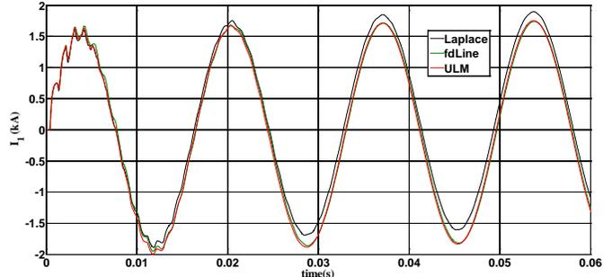
Fig. 38. Detail of current at shorted conductor 1 of two parallel horizontal lines.
