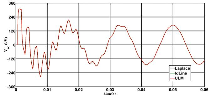
Fig. 8: Voltage at receiving-end of open single-phase line.
