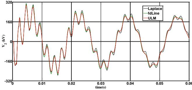
Fig. 35. Detail of voltage at open conductor 2 of two parallel horizontal lines.
