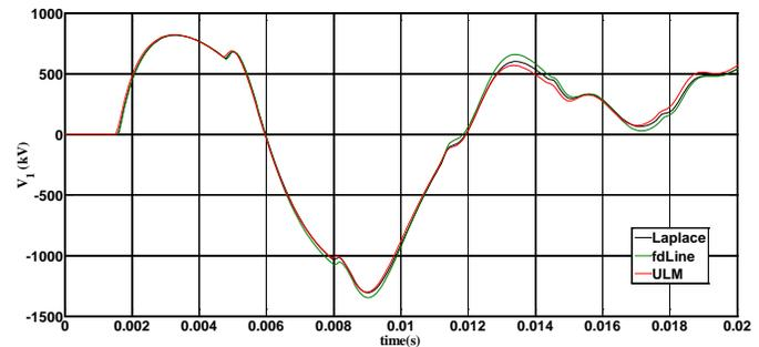
Fig. 24. Further detail of voltage at open conductor 1 of delta line.
