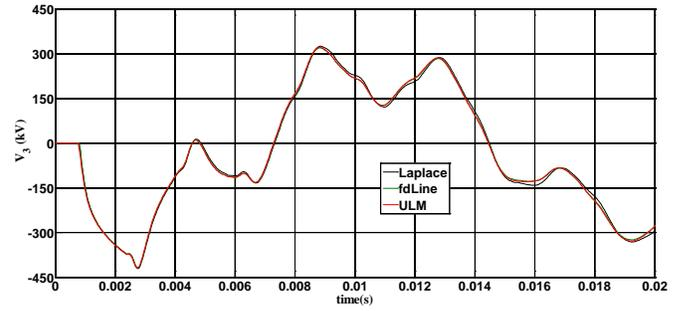
Fig. 12. Further detail of voltage at open conductor 3 of horizontal line.
