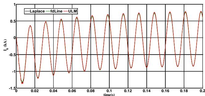
Fig. 31. Current at shorted conductor 6 of double-circuit one-tower delta line.
