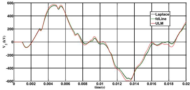
Fig. 18. Further detail of voltage at open conductor 2 of vertical line.
