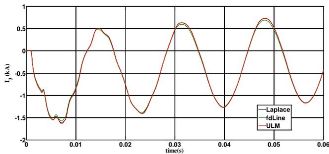
Fig. 20. Detail of current at shorted conductor 3 of vertical line.
