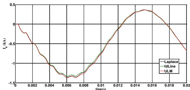
Fig. 33. Further detail of current at shorted conductor 6 of double-circuit one-tower delta line.
