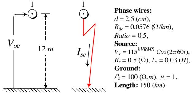
Fig. 1. Single-phase transmission line (open and shorted). ( $\Delta t = 5 \mu s$ )
