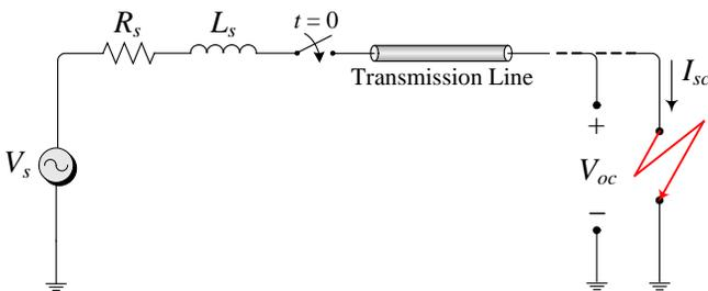
Fig. 7: One-line diagram of the equivalent circuit for the tests.
