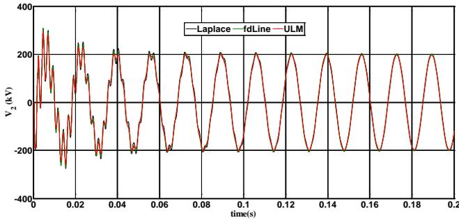
Fig. 34. Voltage at open conductor 2 of two parallel horizontal lines.
