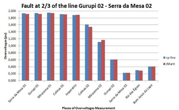
Fig. 9. Peak voltage profile along the AC-Link considering a three-phase fault at 2/3 of the length of the line Gurupi 2 – Serra da Mesa 2.
