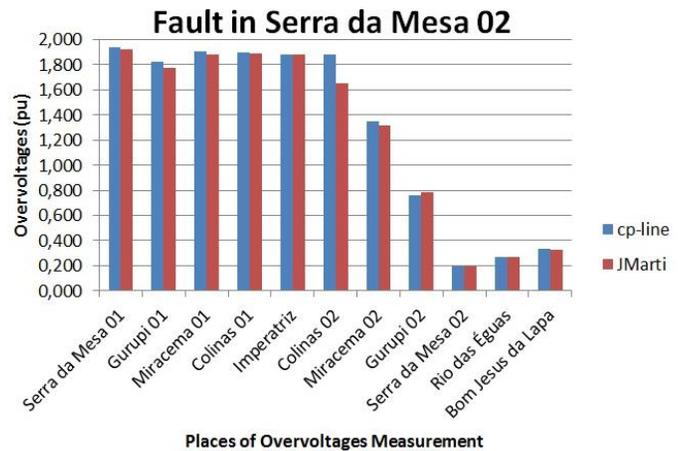
Fig. 10. Peak voltage profile along the AC-Link considering a three-phase fault in Serra da Mesa 2.
