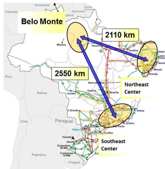
Fig. 1. Distances from the generation in the Amazon region to the main load centers in the Southeast and Northeast.
