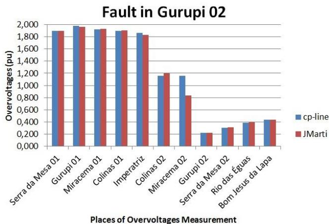
Fig. 7. Peak voltage profile along the AC-Link considering a three-phase fault in Gurupi 2.
