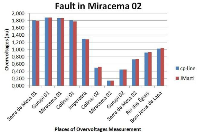
Fig. 4. Peak voltage profile along the AC-Link considering a three-phase fault in Miracema 2.
