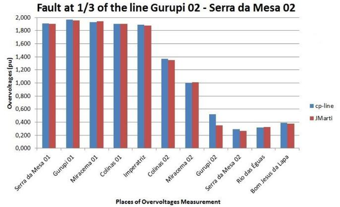
Fig. 8. Peak voltage profile along the AC-Link considering a three-phase fault at 1/3 of the length of the line Gurupi 2 – Serra da Mesa 2.
