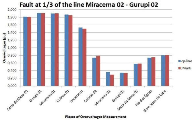
Fig. 5. Peak voltage profile along the AC-Link considering a three-phase fault at 1/3 of the length of the line Miracema 2 – Gurupi 2.
