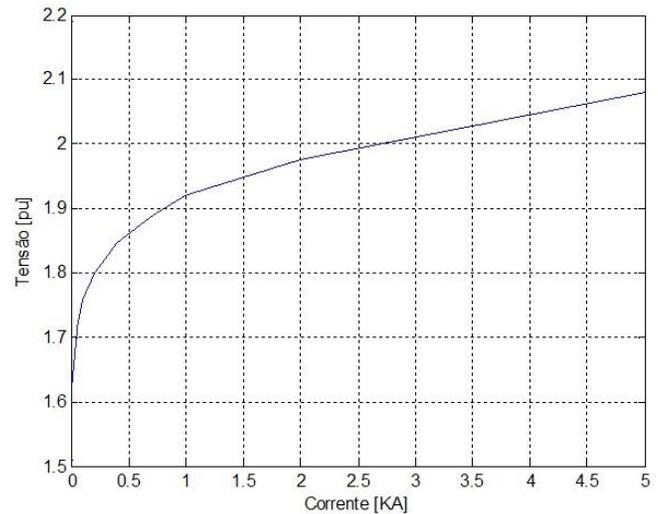
Fig. 3. Characteristic curve of the surge arresters.
