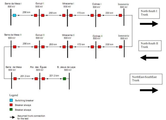
Fig. 2. One line diagram of the AC-Link simulated.
