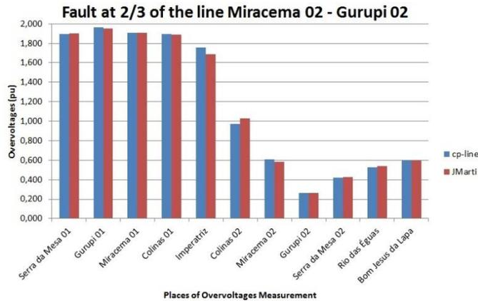
Fig. 6. Peak voltage profile along the AC-Link considering a three-phase fault at 2/3 of the length of the line Miracema 2 – Gurupi 2.
