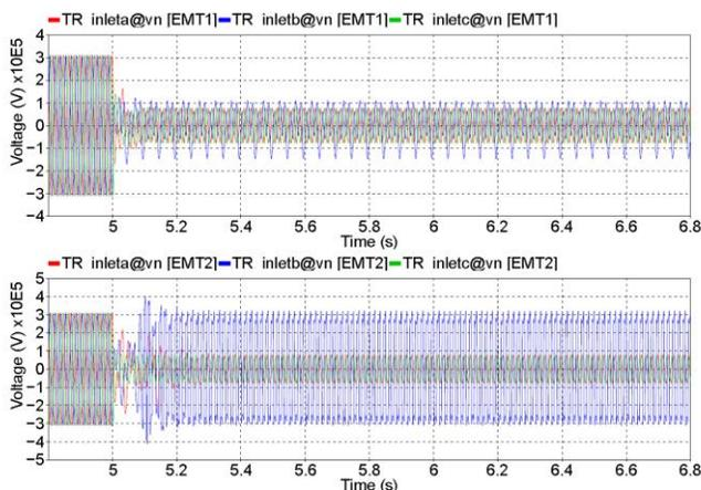
Fig. 15. Voltages at transformer primary side for Case 3 (upper) and Case 4 (lower).
