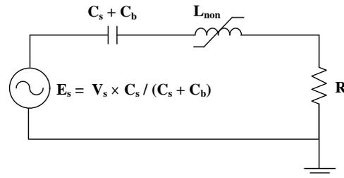
Fig. 5. Equivalent circuit of series non-linear resonance circuit
