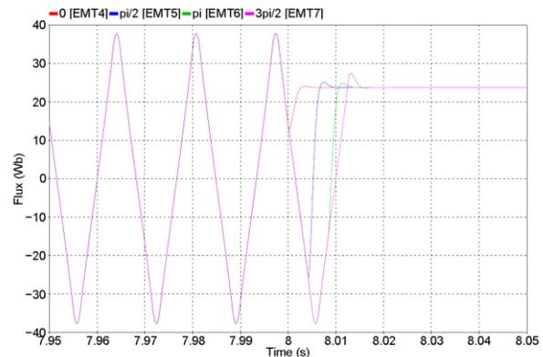
Fig. 18. Variation of residual flux depending on opening instant (Switching instant: red-0, blue-  $\pi/2$ , green- $\pi$ , pink-  $3\pi/2$ ).
