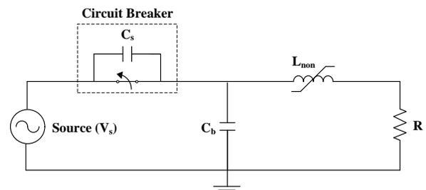
Fig. 2. Series non-linear resonance circuit.
