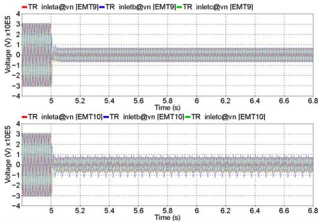
Fig. 14. Voltages at transformer primary side for Case 1 (upper) and Case 2 (lower).
