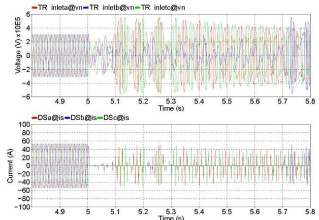
Fig. 9. Voltages at transformer primary side (upper) and line currents (lower) for transformer saturation.
