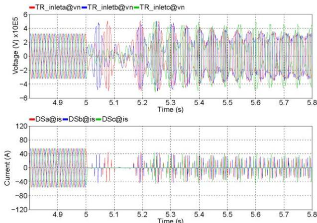
Fig. 4. Voltages at transformer primary side (upper) and line currents (lower) for simulation model.
