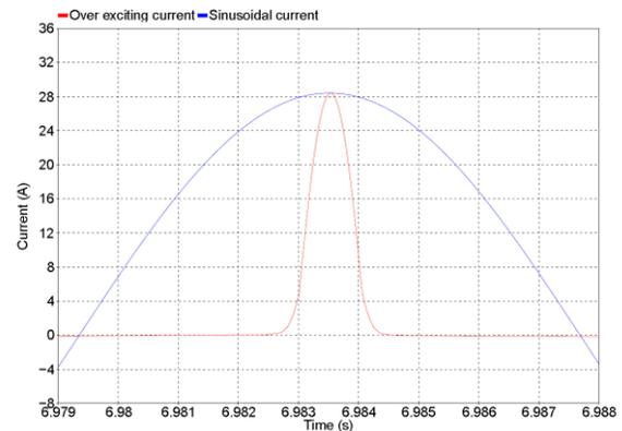
Fig. 16. Enlarged view of over exciting current for basic case together with the sinusoidal current
